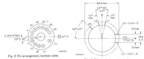
Fig. 4 Side-contact arrangement, bottom view.
