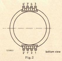
With  $L_3$  and  $L_4$  connected in series as in Fig.3 a current in the direction indicated will produce a clockwise rotation of the vertical trace and an anti-clockwise rotation of the horizontal trace.
