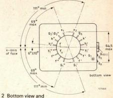
Fig. 2 Bottom view and side-contact arrangement.
