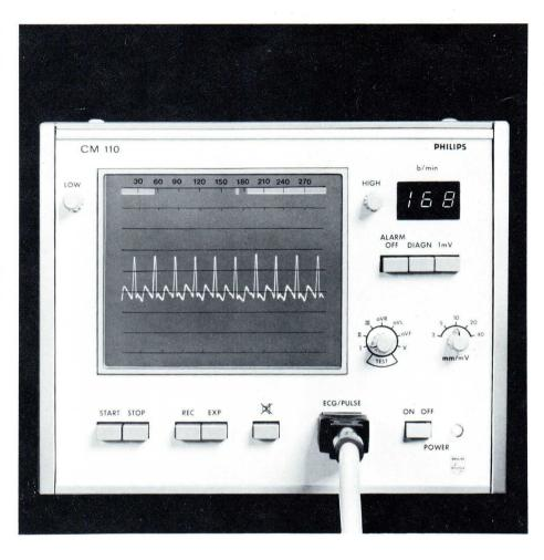
Pacemaker pulses are clearly visible on the cardioscope. In most circumstances they are not counted by the rate counting circuitry. The amplifier is fully defibrillator-proof. Even when defibrillation is done with the electrodes in contact with the ECG electrodes, the apparatus will not be damaged.
