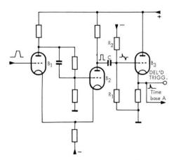
10. Pulse shaper and its associated circuits
