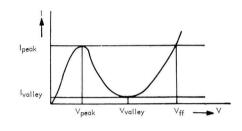
17. Tunnel diode characteristic
