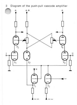
In the AC position of the AC/DC switch large capacitors are included in the feed back circuit. The amplification of very low frequency signals, and also the drift, is now very low. The result is that the drift in the AC positions, caused primaraly by section I, is approximately a factor of one hundred smaller than in the DC positions of the AC/DC switch.
