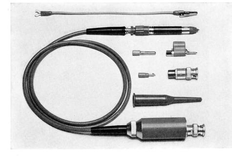
$C_k.$  With  $R_2=1~M\Omega$  and  $C_2=15~pF$  (normal values for input resistance and capacitance of the oscilloscope respectively),  $C_k=30~pF$  (cable length of about 1 m) and  $R_1=9~M\Omega$ , the value of  $C_1$  will be about 5 pF.
