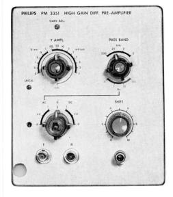
The PM 3351 is a sensitive LF vertical plugin unit, 100  $\mu$ V (200 kHz), which is used in conjunction with the basic oscilloscope PM 3330. The PM 3351 consists of three amplifier sections (see fig. 1).
