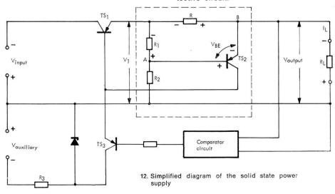
The overload protection circuit consists basically of the transistor  $TS_2$  and resistors R,  $R_1$  and  $R_2$  as shown in the simplified diagram. Under normal working conditions load resistance  $R_L = R_{nom.}$ , point A is positive with respect to point B, and  $TS_2$  is cut-off. Thus the voltage comparator circuit is able to exercise full control of the series regulator transistor  $TS_1$  via emitter follower  $TS_2$
