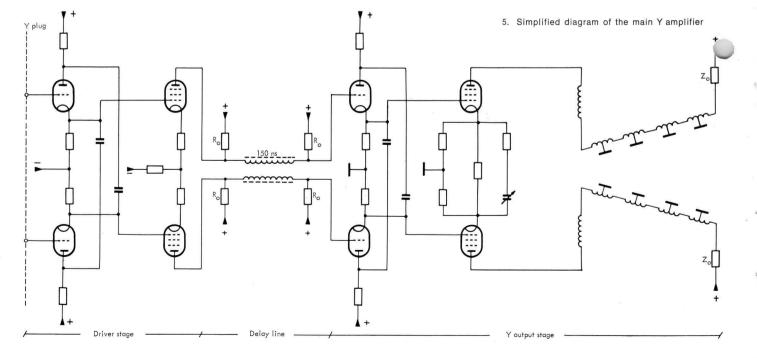
The input impedance  $Z_i$  then equals  $R_0$  thus  $Z_i$  is independent of frequency. The voltage transfer to the deflection
