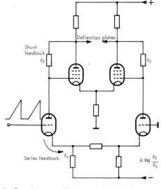
9. Paraphase amplifier as used in the X output stage
