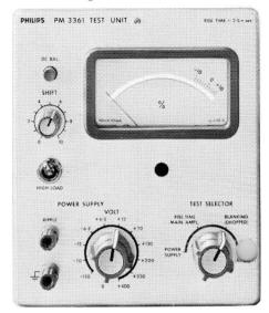
This plug-in facilitates testing of the main frame, output amplifier, power unit and blanking circuit. It provides:
