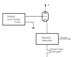
16. Simplified diagram of the calibration unit
