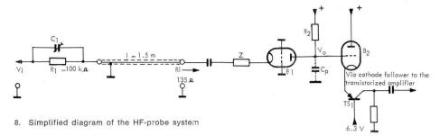
With  $R_1' = 100 \ k\Omega$ ,  $R_2' = 33 \ k\Omega$ , and  $C_2' = 9 \ pF$ , the value of C1' will be about 3 pF. The input capacitance including the parasitic capacitance measured at the tip of the probe, will now be about 5 pF.
