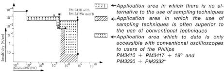
ternative to the use of sampling techniques Application area in which the use of sampling techniques is often superior to the use of conventional techniques ← Application area which to date is only
