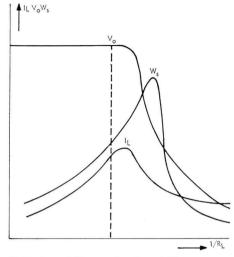
14.  $V_0$ ,  $I_L$  and  $W_s$  as a function of  $^{1}/R_L$
