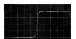
Overall step response of the amplifier; rise time of the input signal amounts to about 1ns, time scale 10 ns/cm
