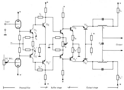
Because of this and the low output resistance of  $TS_2$  the preamplifier stage has a wide bandwidth. For a detailed treatment of this circuit, reference is made to the articles written by Dr. Cherry and Mr. Hooper, of the Department of Electrical Engineering, University of Melbourne.\*
