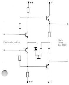
4. Circuit diagram of the final stage
