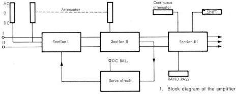
automatic control adjustment of the amplifier DC balance.
