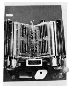
Cooling unit, with power transistors, can be taken out and interconnected with the apparatus by means of a connector block. The transistors on this cooling unit are then interchangeable. Special holder for the transistors renders soldering unnecessary
