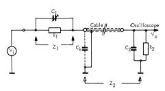
5. Principle of the passive probe
