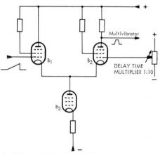
9. Voltage comparator circuit
