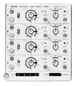
The PM 3344 is a four trace unit for oscilloscope PM 3330. With this unit four signals can be displayed simultaneously. Moreover there is the possibility of changing the polarity of each channel or simply be switching it off.
