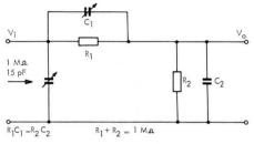
ductance of the capacitors and the earth connections, begin to play a role. In this way the attenuation becomes dependent on the frequency which, in pulse reproduction leads to distortion of the flanks. A great deal of care has therefore been devoted to the attenuator used in the PM 3333, with respect to good high-frequency earthing, and special HF disc capacitors of very low self-inductance have been incorporated.
