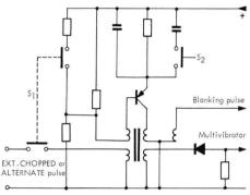
5. Circuit diagram of blocking oscillator
