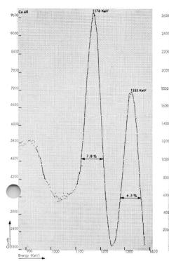
Co<sup>60</sup> spectrum recorded with a conventional single crystal spectrometer consisting of a 1<sup>3</sup>/<sub>4</sub>" diameter x 2" thick Nal (TI) crystal coupled to a 2" photomultiplier tube
