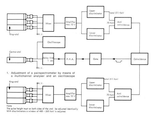
A special gamma radiation spectrometer is described, which has several advantages over the conventional single crystal spectrometer. These advantages are:
