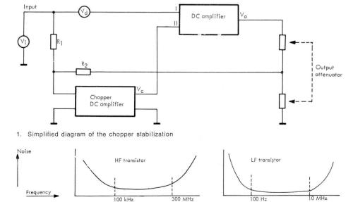
Thus it can be seen that while the input signal V<sub>i</sub> benefits from the full amplification A of the DC amplifier the drift voltage is only amplified  $A/(1+^{1}/_{2}B)$  where B is in the order of several thousands. In this way the drift is greatly reduced. It should be noted that this method of chopper stabilization has no effect on the input impedance as the junction of R<sub>1</sub> and R<sub>2</sub> is a virtual earth point in relation to the input signal.
