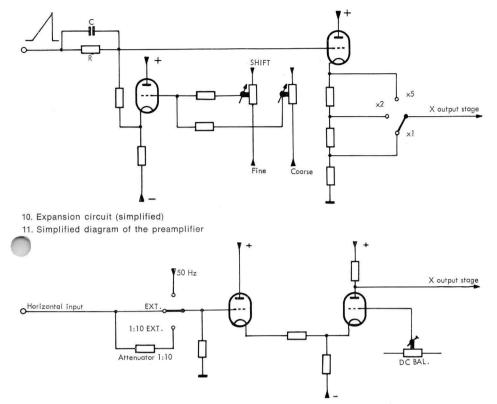
terminal. When the mode switch is at EXT. this signal is amplified by a preamplifier (fig. 11), and used to drive the X output stage. For large input signals a 1:10 attenuator can be interposed between the signal and the preamplifier.
