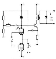
6. Simplified diagram of the trigger unit with tunnel diode
