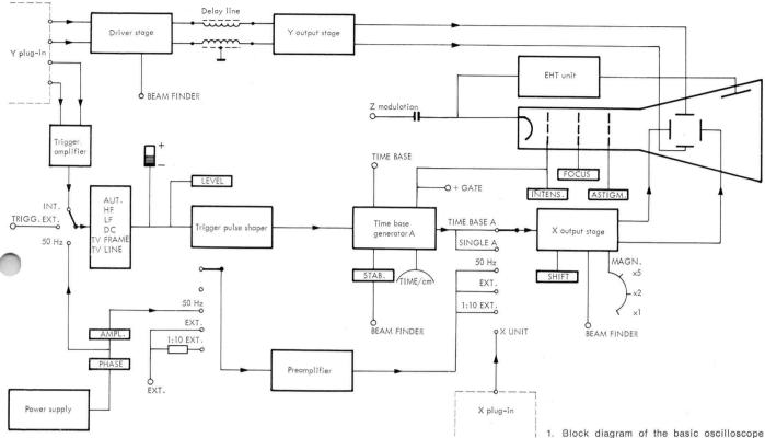
Philips cathode-ray oscilloscope The PM 3330 is a 60 MHz instrument which has a wide range of applications. This is achieved by the utilization of plug-in units, each of which covers one or more fields of application. Plug-in units are available both for the Y and the X channels.
