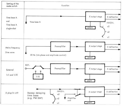
Survey of functions of the horizontal amplifier circuit
