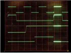
Here the main time base has been changed to channel B and the delayed to channel B. The two differentials can also be shown or displayed separately. Dual X-Y displays are yet another example of the PM 3244's remarkable display versatility.
