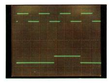
simultaneously, however, gives the logic sequence at a glance and without error. It is also much more meaningful. The PM 3244 is thus ideal for a wide range of 'parallel' applications: coding and decoding systems, for example, where several inputs and one or more outputs need to be checked: the address, read, write and strobe signals in memories and for checking the data contents of several tracks of tape or disk memories.
