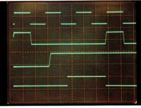
As illustrated, triggering is fully independent and multi-sourced. Main and delayed time bases can be triggered from any of the four signals plus Composite. The main time base can also be triggered on External and Line.
