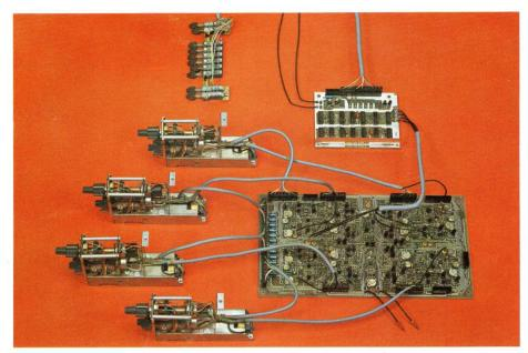
The main amplifier pannel of the PM 3244 is Electrically connected to front pannel controls and simple DC signals are used to change operating parameters.
