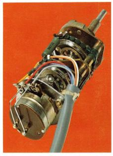
A dramatic simplication of the main time base switch as a result of cold switching techniques.
