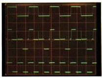
Three traces illustrating differential display facilities. In this case a simultaneous display of channel A,-B and A-B. The identical facility exists for C and D channels.
