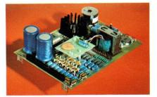
Direct conversion power supply as used on PM 3244.
