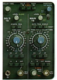
The main and delayed time base controls are separed in order to avoid ambiguity and possible errors. The controls are on the same level as those of the Y channels but clearly distinguishable. Note also that the vernier control of delay time is positioned so that the setting cannot be accidentally changed.
