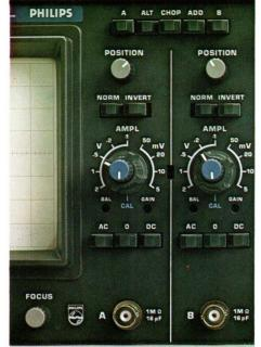
The front panel of the PM 3200 has been designed to an extremely high ergonomic standard. Both Y channels, for example, are logically grouped together, but clearly distinguishable. Note too the wide choice of display modes – chopped and alternate, with normal and inverted positions for both channels.
