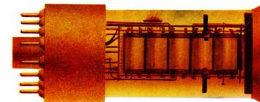
shown in the figures in this folder. It is recommended to use a bleeder current of at least 100 times the average anode current of the photomultiplier. In pulse techniques, such as scintillation counting, a bleeder current of about 1 mA is usually sufficient, provided that the last two or three stages are decoupled by means of capacitors of 100 pF and 200 pF.
