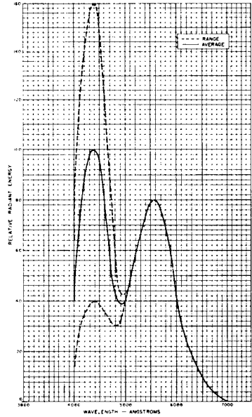
Spectral-Energy Emission Characteristic of Phosphor P7
