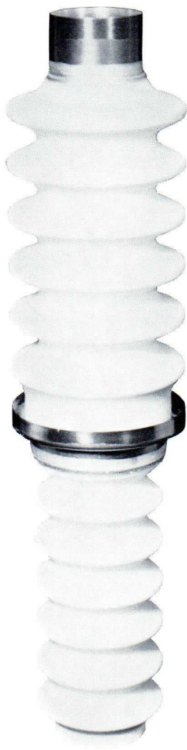
Typical 100 kV terminal in the PTC 1080 series with alumina ceramic corrugated for increased dielectric path.
