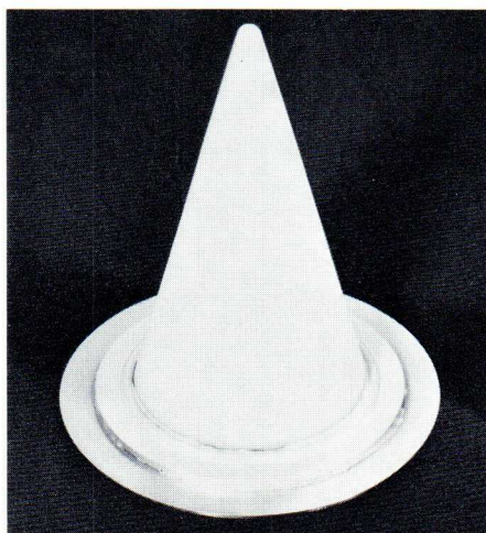
PTC 1100, one of the range of EMI-Varian high power microwave windows. The material is Al_2O_3 (98.5%). Sealed via Vacon 70 to Nilo-k.
