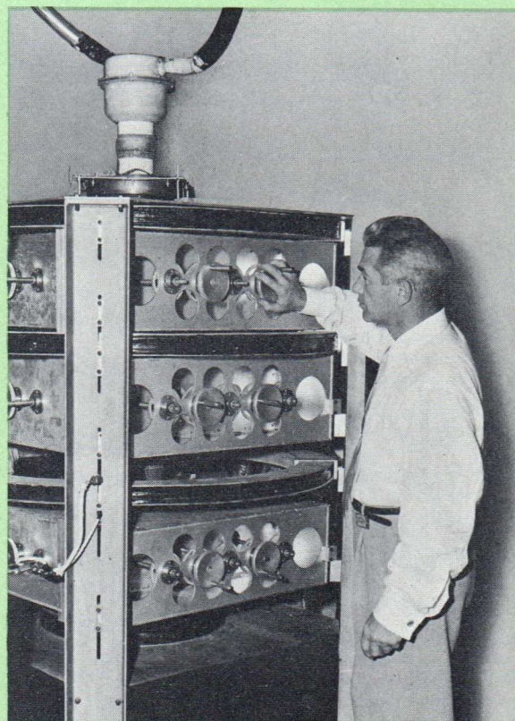
Figure 9 Eimac X590D amplifier klystron and circuit components
