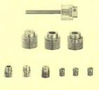
Eimac Preformed Finger Stock is a prepared strip of spring material slotted and formed into a series of fingers designed to make a sliding contact. It is especially suitable for making connections to tubes with coaxial terminals or to moving parts, such as long-line and cavity circuits or screen-room doors. Eimac finger stock is available in 9 dif-
