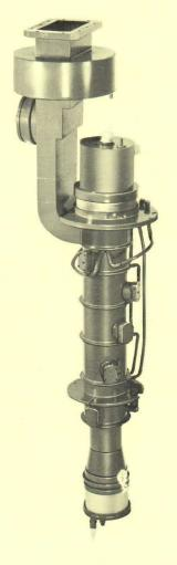
The X832 pulse amplifier klystron, shown here, is an example of Eimac's leadership in the pulse field. Due to the use of a high perveance hollow beam this tube produces 12% bandwidth and a peak output power of 10 Mw with peak beam voltage of only 114 kilovolts.
