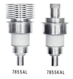
In addition to these features, these tubes also incorporate the arc-resistant cathode which assures stable operation under adverse conditions and which minimizes catastrophic failures due to arc-over during circuit malfunction. These tubes are useable from dc to 3 GHz.
