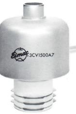
The 3CV1500A7 is an integral-boiler, ceramic/metal, vapor cooled zerobias triode, intended for Class AB2 linear amplifier service in either grid driven or cathode driven configuration. Except for the anode dissipation rating, the 3CV1500A7 is electrically identical to the EIMAC 8283/3CX-1000A7.
