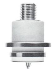
The Y-690 is an 8941 which has been specially processed for series regulator and switch tube service and will operate in some applications to 15 KV<sup>1</sup>. Solder tabs are available on special request permitting attachment of flying leads for grid, cathode and heater connections.
