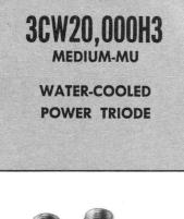
The Eimac 3CW20,000H3 is a water-cooled, ceramic-metal power triode designed primarily for use in industrial radio-frequency heating services. Its water-cooled anode is conservatively rated at 20 kilowatts of plate dissipation with low water flow and pressure drop.
