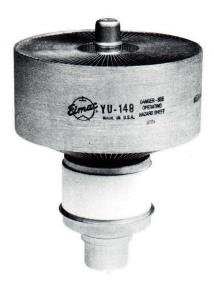
The EIMAC YU-148 high mu, forced air cooled, power triode provides relatively high power output as an amplifier, oscillator or modulator at low plate voltages. The tube has a low inductance cylindrical filament stem structure which readily becomes part of a linear filament tank circuit for VHF operation. The grid provides good shielding between the input and output circuits for grounded grid applications and conveniently terminates in a ring between the plate and filament terminals.
