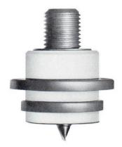
The 8940 is normally supplied without a radiator and may be conduction, convection, heatsink, or liquid cooled. Liquid cooling can be done by submersion of the tube in an insulating medium such as FC-75. Radiators for forced-air cooling as well as heat-sink adaptors permitting anode dissipation up to 750 watts are available as separate items.
