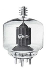
The EIMAC 8163/3-400Z is a compact power triode intended to be used as a zero-bias Class-B amplifier in audio or radio-frequency applications. Operation with zero grid bias simplifies associated circuitry by eliminating the bias supply. In addition, grounded-grid operation is attractive since a power gain as high as twenty times can be obtained with the 8163/ 3-400Z in a cathode-driven circuit.
