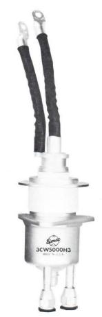
The EIMAC 3CW5000H3 is a water-cooled, ceramic-metal power triode designed primarily for use in industrial radio-frequency heating services. Its water-cooled anode is conservatively rated at 5 kilowatts of plate dissipation with low water flow and pressure drop.
