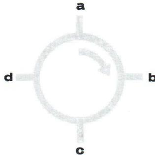
Huggins Ferrite Circulators are non-reciprocal microwave networks which transmit power from one terminal to another in sequence. Power introduced at port "a" leaves the network at port "b"... "b" at "c"... "c" at "d"... and "d" at "a". These Ferrite Circulators provide an entirely new parameter for the design of microwave circuits.
