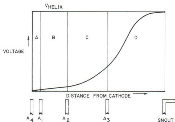
FIGURE 1. POTENTIAL PROFILE AND RELATIVE POSITION OF THE ELECTRODES IN A TYPICAL MULTI-REGION LOW-NOISE ELECTRON GUN.
