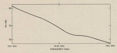
SMALL SIGNAL GAIN VS FREQUENCY -10 dB BELOW SATURATION
