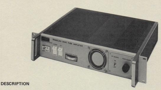
The Hughes Model 1216H RF generator is tunable across the frequency range at 3.0 to 3.5 GHz with a minimum of 10 watts of RF power output. Each generator consists of a PPM metal-ceramic traveling-wave tube, a regulated solid-state power supply and complete
