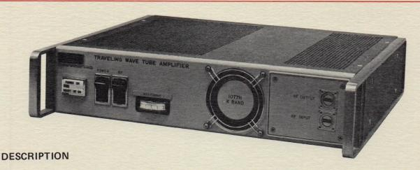
The Hughes Model 1077H11 Traveling-Wave Tube Amplifier provides a minimum power output of 1 watt over the 18 – 26.5 GHz frequency range. The amplifier consists of a Hughes PPM metal-ceramic traveling-wave tube, a regulated solid state power supply and complete air cooling system assembled within a compact instrument case.
