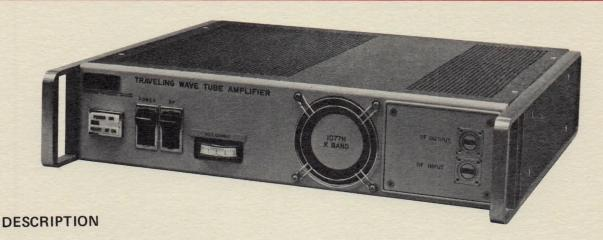
The Hughes Model 1077H11 Traveling-Wave Tube Amplifier provides a minimum power output of 1 watt over the  $18-26.5\,\mathrm{GHz}$  frequency range. The amplifier consists of a Hughes PPM metal-ceramic traveling-wave tube, a regulated solid state power supply and complete air cooling system assembled within a compact instrument case.
