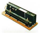
Model 1288H Space qualified traveling-wave tube amplifier. Includes electronic power conditioner, TWT, and interface circuitry in a light weight (3.75 pounds) package. This 5W, 4 GHz TWTA has a design life of seven years. Forty-eight of the amplifiers are currently in orbit providing domestic communication service.
