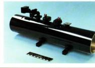
Model 876H TWT. 700 watt coupled cavity traveling-wave tube at 14.0 to 14.5 GHz. A PPM focused, air cooled TWT for satellite earth terminals. Efficiency greater than 40%. Consertive design and dual ion pumps insure long operational and shelf life.
