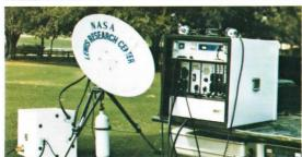
(above) A 14 GHz power amplifier provides 20 Watts of RF output for this transportable terminal. The small power amplifier is housed in a weatherized housing adjacent to the antenna and controlled in a remote panel.
