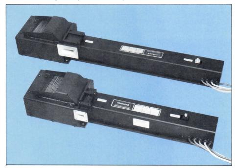
**Figure 64** — Models 662H & 881H 250 and 400 watt helix traveling-wave tubes used in commercial earth terminals at 6 and 14 GHz. Both are PPM-focused, air-cooled, and compatible with a single power supply design.
