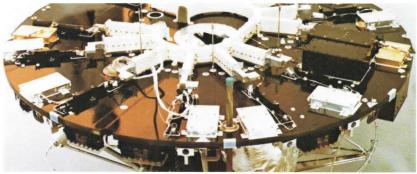
**Satellite Transponder Shelf** Space qualified traveling wave tubes and amplifiers mounted on the communication shelf of a typical domestic satellite.
