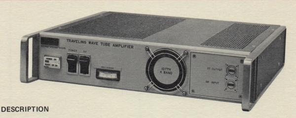
The Hughes Model 1077H12 Traveling-Wave Tube Amplifier provides a minimum power output of 1 watt over the 26.5-40 GHz frequency range. The amplifier consists of a Hughes PPM metal-ceramic traveling-wave tube, a regulated solid state power supply and complete air cooling system assembled within a compact instrument case.
