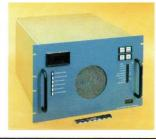
Model 1273H. Electronic Power Conditioner (EPC) offers special controls and logic interfaces for 14 GHz RF terminals. TWT voltages are programmed by the tubes permitting field replacement without power supply adjustment. This three phase, 2 KVA power supply weighs less than 85 pounds.
