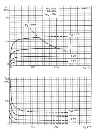
ANODE AND SCREEN-GRID CURRENTS PLOTTED AGAINST ANODE VOLTAGE WITH CONTROL-GRID VOLTAGE AS PARAMETER, V  $_{\rm g2}$  = 75V. F SECTION
