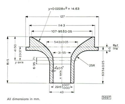
REFERENCE LINE GAUGE J.E.D.E.C. 126 FOR MONOCHROME CATHODE RAY TUBES HAVING 110° SCANNING ANGLES AND A NECK DIAMETER OF 28-6mm
