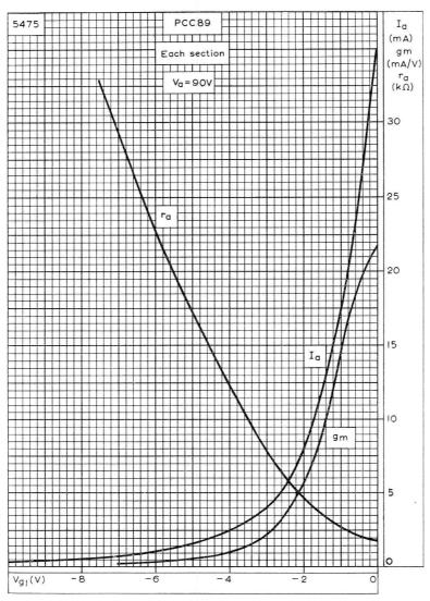
ANODE CURRENT, MUTUAL CONDUCTANCE AND ANODE IMPEDANCE
