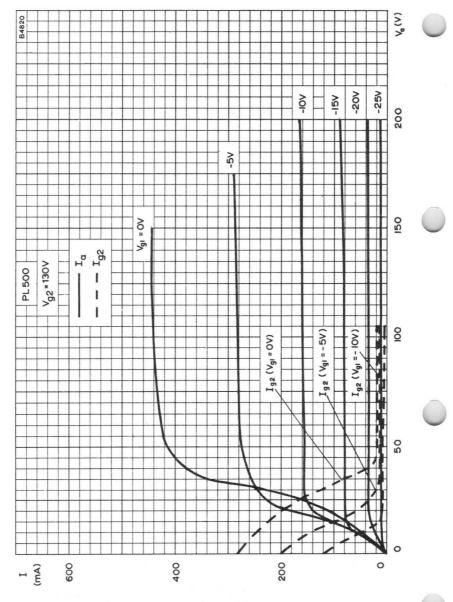
ANODE AND SCREEN CURRENTS PLOTTED AGAINST ANODE VOLTAGE WITH CONTROL-GRID VOLTAGE AS PARAMETER. V  $_{\rm g2}$  = 130V
