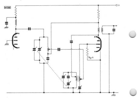
OPERATING CONDITIONS AS SELF-OSCILLATING ADDITIVE MIXER (with i.f. feedback, see basic circuit in fig.1.)
