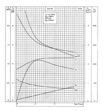
PERFORMANCE CURVES FOR USE AS FREQUENCY CHANGER WITH  $R_{\textbf{k}}{=}0\Omega$
