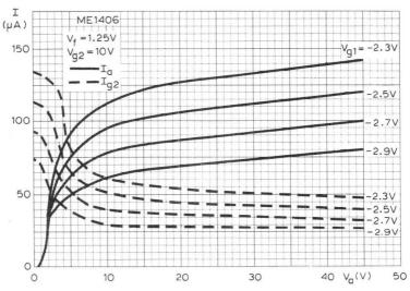
ANODE AND SCREEN-GRID CURRENTS PLOTTED AGAINST ANODE VOLTAGE WITH CONTROL-GRID VOLTAGE AS PARAMETER. V  $_{\rm g2}$  = 10V.
