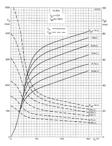
ANODE AND SCREEN CURRENTS PLOTTED AGAINST ANODE VOLTAGE
