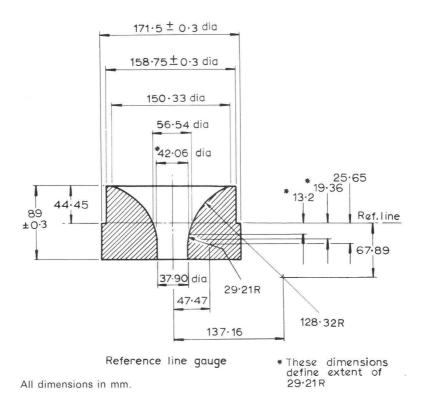
REFERENCE LINE GAUGE FOR COLOUR CATHODE RAY TUBES HAVING 90° SCANNING ANGLES AND A NECK DIAMETER OF 36.5mm
