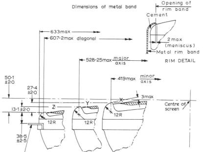
One of the four lugs may deviate 2mm max. from the plane through the three other lugs. This deviation is incorporated in the  $\pm 2 \cdot 5$  tolerance.
