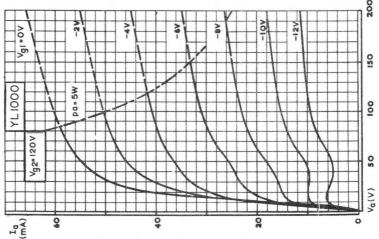
anode current plotted against anode voltage with control-grid voltage as parameter  $\rm V_{\rm g2}{=}120V$
