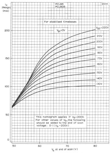
DESING CHART FOR STABILISED TIME BASES: PENTODE SECTION
