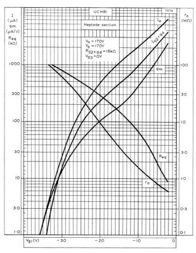
ANODE AND SCREEN-GRID CURRENTS, MUTUAL CONDUCTANCE, ANODE IMPEDANCE, AND EQUIVALENT NOISE RESISTANCE PLOTTED AGAINST CONTROL-GRID VOLTAGE FOR HEPTODE SECTION.  $V_a = 170 \text{V} \label{eq:value}$
