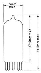
The bulb and base dimensions of this valve are in accordance with BS448, Section B7G
