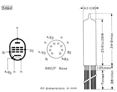
The bulb and base dimensions of this valve are in accordance with BS448, Section B8D/F.
