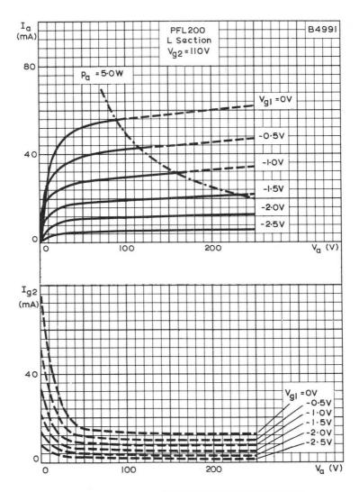
ANODE AND SCREEN-GRID CURRENTS PLOTTED AGAINST ANODE VOLTAGE WITH CONTROL-GRID VOLTAGE AS PARAMETER. V  $_{\rm g2}$  = 110V. L SECTION
