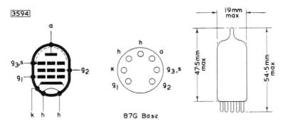
The bulb and base dimensions of this valve are in accordance with BS448, Section B7G
