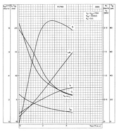
PERFORMANCE CURVES FOR USE AS A FREQUENCY CHANGER WITH  $R_{\rm k} = 0 \Omega \label{eq:reconstruction}$
