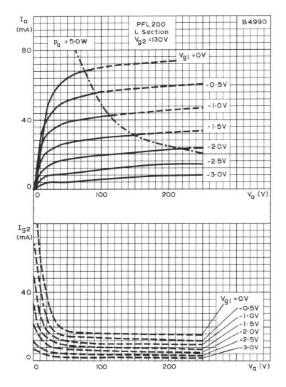
ANODE AND SCREEN-GRID CURRENTS PLOTTED AGAINST ANODE VOLTAGE WITH CONTROL-GRID VOLTAGE AS PARAMETER. V  $_{\rm g2}$  = 130V. L SECTION
