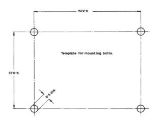
The bolts to be used for mounting the tube must be within the circles of 9-5mm diameter shown in the template drawing.
