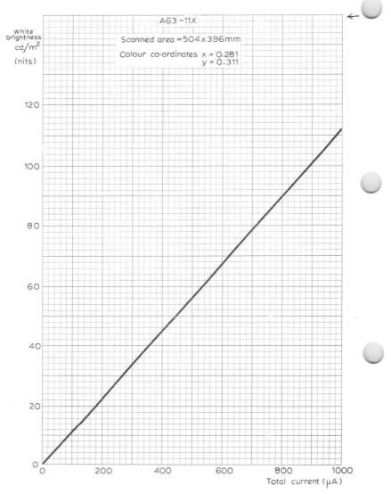
BRIGHTNESS AT CENTRE OF SCREEN AS A FUNCTION OF TOTAL CURRENT FOR WHITE OF COLOUR COORDINATES  $x=0.281,\ y=0.311$
