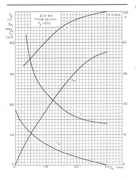
AMPLIFICATION FACTOR, MUTUAL CONDUCTANCE, ANODE IMPEDANCE AND CONTROL-GRID VOLTAGE PLOTTED AGAINST ANODE CURRENT.  $V_a = 50 \text{V. TRIODE SECTION} \label{eq:vactor}$
