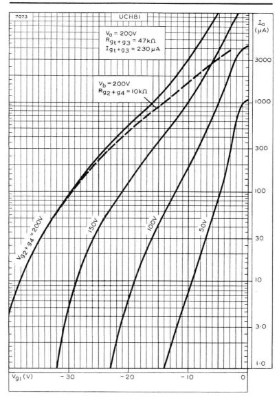
ANODE CURRENT PLOTTED AGAINST CONTROL-GRID VOLTAGE WHEN USED AS FREQUENCY CHANGER.  $V_a = 200 \text{V} \label{eq:value}$
