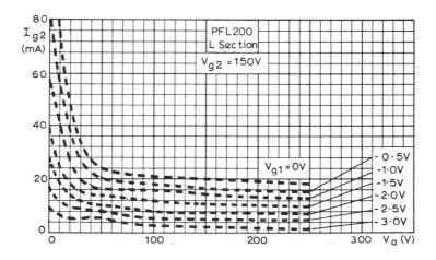
ANODE AND SCREEN-GRID CURRENTS PLOTTED AGAINST ANODE VOLTAGE WITH CONTROL-GRID VOLTAGE AS PARAMETER. V  $_{\rm g2}$  = 150V. L SECTION
