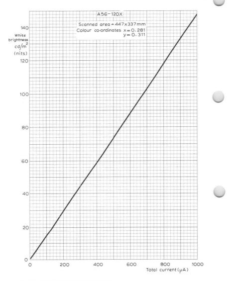
BRIGHTNESS AT CENTRE OF SCREEN PLOTTED AGAINST TOTAL CURRENT FOR WHITE OF COLOUR COORDINATES x=0.281, y=0.311
