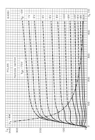
ANODE CURRENT PLOTTED AGAINST ANODE VOLTAGE WITH CONTROLGRID VOLTAGE AS PARAMETER. V  $_{\rm g2}$  = 170V. PENTODE SECTION
