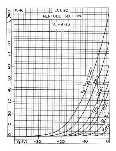
ANODE CURRENT OF PENTODE SECTION PLOTTED AGAINST CONTROL-GRID VOLTAGE, FOR ANODE AND SCREEN-GRID VOLTAGES BETWEEN 50V AND 300V
