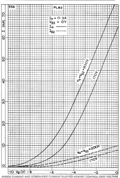
Video output pentode for use in television receivers with series connected heaters. It is particularly suitable for use in projection television receivers or with high definition television systems.
