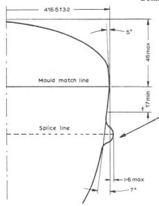
†Undisturbed area between mould match line and splice line
