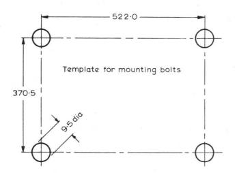
The bolts to be used for mounting the tube must be within the circles of 9.5mm diameter shown in the template drawing.
