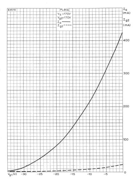
ANODE AND SCREEN CURRENTS PLOTTED AGAINST CONTROL-GRID  ${\tt VOLTAGE }$
