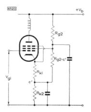
With compensating resistor Rk1 (e.g. vision i.f. amplifier)
