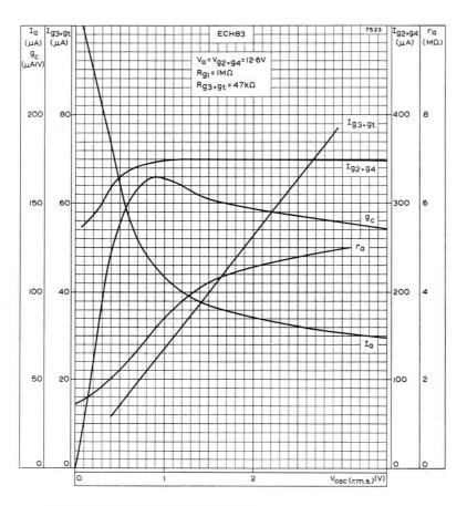
PERFORMANCE CURVES FOR USE AS A FREQUENCY CHANGER  $V_a = V_{\rm g2+g4} = 12.6 \text{V}$
