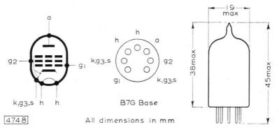
The bulb and base dimensions of this valve are in accordance with BS448, Section B7G
