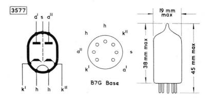
Double diode with separate cathodes and internal screening between sections.
