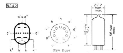
The triode on pins 6, 7, 8, should have the grounded cathode connection and that on pins 1, 2, 3, should have the grounded grid connection.
