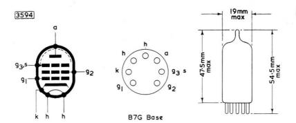
The bulb and base dimensions of this valve are in accordance with BS448 Section B7G
