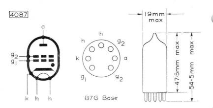
The bulb and base dimensions of this valve are in accordance with BS 448, Section B7G
