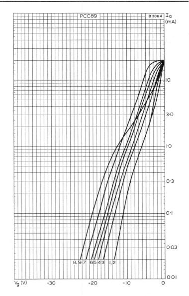
ANODE CURRENT PLOTTED AGAINST CONTROL-GRID VOLTAGE UNDER CONDITIONS 1 to 9 (See page D3)
