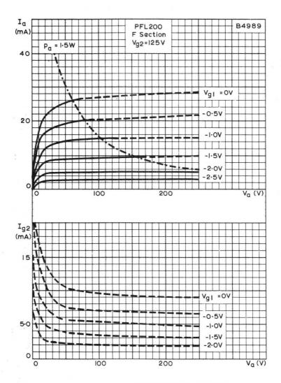
ANODE AND SCREEN-GRID CURRENTS PLOTTED AGAINST ANODE VOLTAGE WITH CONTROL-GRID VOLTAGE AS PARAMETER. V  $_{\rm g2}$  = 125V. F SECTION
