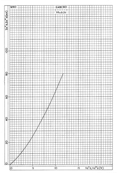
ANODE CURRENT PLOTTED AGAINST ANODE VOLTAGE FOR DIODE SECTIONS  $a^{\prime\prime}{}_d$  AND  $a^{\prime\prime\prime}{}_d$
