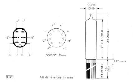
The bulb and base dimensions of this valve are in accordance with BS448, Section B8D/F  $\,$
