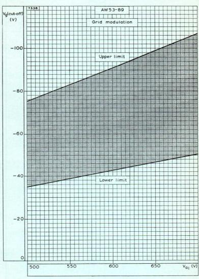
LIMITS OF GRID CUT-OFF VOLTAGE FOR FIRST ANODE VOLTAGES OF 500V to 700V. GRID MODULATION
