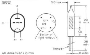
Connections should not be soldered nearer than 5mm from the seal. The leads should not be bent nearer than 1.5mm from the seal.
