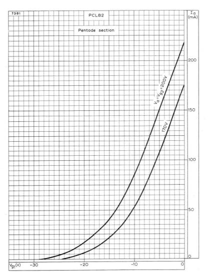
ANODE CURRENT PLOTTED AGAINST CONTROL-GRID VOLTAGE WITH ANODE AND SCREEN-GRID VOLTAGES AS PARAMETER, PENTODE SECTION
