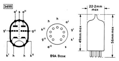
The bulb and base dimensions of this valve are in accordance with BS448 Section B9A
