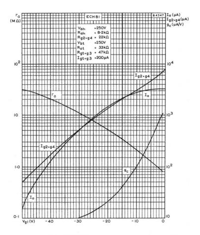
ANODE AND SCREEN-GRID CURRENTS, CONVERSION CONDUCTANCE
