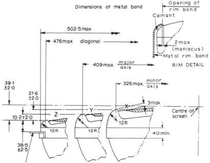
One of the four lugs may deviate 2mm max. from the plane through the three other lugs This deviation is incorporated in the  $\pm\,2\cdot5$  tolerance.
