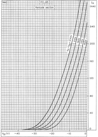
ANODE CURRENT PLOTTED AGAINST CONTROL-GRID VOLTAGE WITH ANODE AND SCREEN-GRID VOLTAGES AS PARAMETER, PENTODE SECTION
