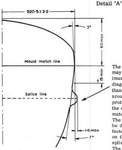
†Undisturbed area between mould match line and splice line
