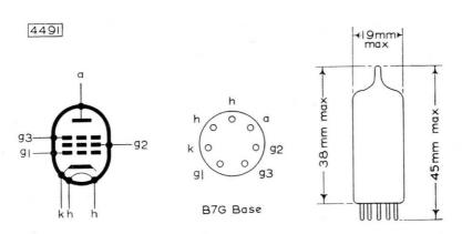
The bulb and base dimensions of this valve are in accordance with BS448, Section B7G.
