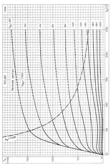
ANODE CURRENT PLOTTED AGAINST ANODE VOLTAGE WITH CONTROLGRID VOLTAGE AS PARAMETER. PENTODE SECTION.  $V_{\rm g2}=170 \rm V$
