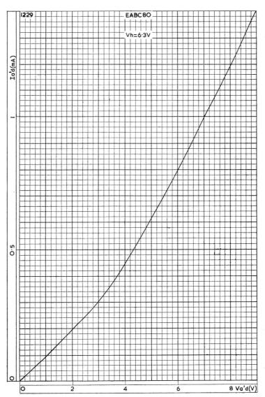
ANODE CURRENT PLOTTED AGAINST ANODE VOLTAGE FOR DIODE SECTION  $a^\prime_d$
