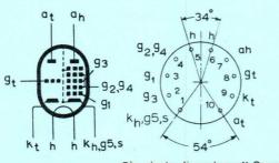
Pin circle diameter = 11.9mm Pin diameter = 1.0mm
