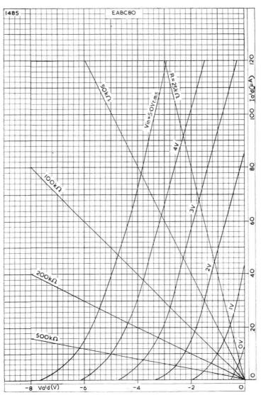
RECTIFIED CURRENT PLOTTED AGAINST OUTPUT VOLTAGE WITH INPUT VOLTAGE BETWEEN 0V AND 5V\_{\rm r.m.s.} AS PARAMETER FOR DIODE SECTION  $a_{\rm rl}^{\prime}$
