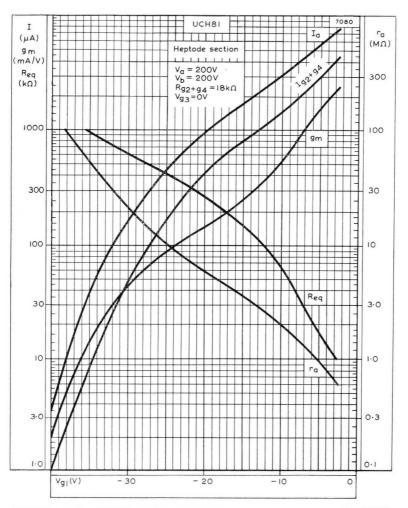
ANODE AND SCREEN-GRID CURRENTS, MUTUAL CONDUCTANCE, ANODE IMPEDANCE, AND EQUIVALENT NOISE RESISTANCE PLOTTED AGAINST CONTROL-GRID VOLTAGE FOR HEPTODE SECTION  $V_a = 200 \text{V} \label{eq:varphi}$
