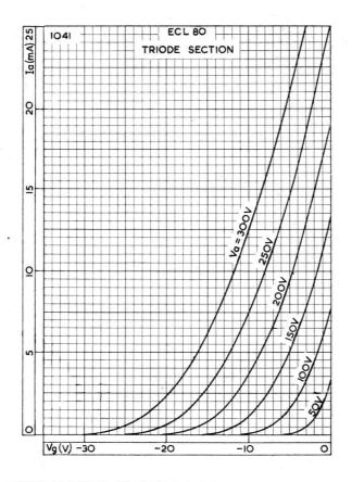
ANODE CURRENT OF TRIODE SECTION PLOTTED AGAINST GRID VOLTAGE, WITH ANODE VOLTAGE AS PARAMETER
