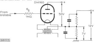
Fig. 2 Digital read-out circuit with DM160 connected to positive logic circuit which uses bistables equipped with n-p-n transistors. The 'High' output level of the bistable may vary between +7.5V and +12V, and the 'Low' level between 0V and +0.4V.  $R_{\rm g}$  protects the valve against excessive anode currents and positive grid currents in case the grid voltage exceeds the cathode potential.
