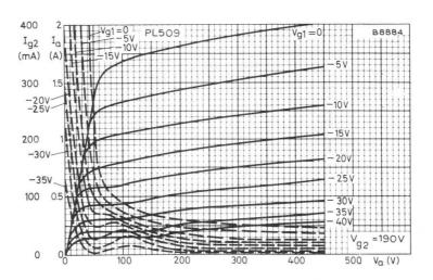
ANODE AND SCREEN GRID CURRENTS PLOTTED AGAINST ANODE VOLTAGE: V  $_{\rm g2} = 190 \rm V$
