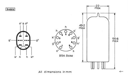
The triode on pins 6, 7, 8 should be used as the r.f. amplifier and that on pins 1, 2, 3 as the self-oscillating additive mixer.
