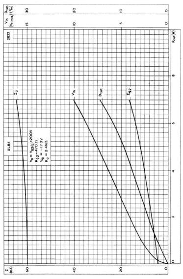
PERFORMANCE OF UL84 WHEN USED AS SINGLE VALVE AMPLIFIER  $V_{\rm a} = V_{\rm g2(b)} = 200 V$
