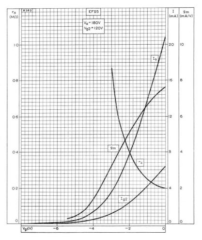
ANODE CURRENT, SCREEN-GRID CURRENT, MUTUAL CONDUCTANCE AND ANODE IMPEDANCE PLOTTED AGAINST CONTROL-GRID VOLTAGE.  $Va = 180 \text{V} \label{eq:value}$
