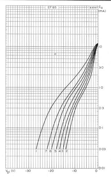
ANODE CURRENT PLOTTED AGAINST CONTROL-GRID VOLTAGE UNDER CONDITIONS 1 to 7 (See page D1)
