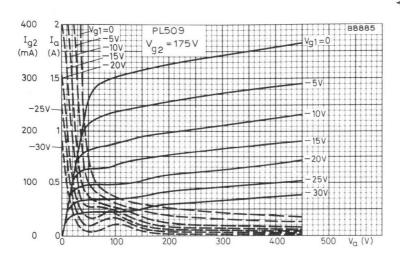
ANODE AND SCREEN GRID CURRENTS PLOTTED AGAINST ANODE VOLTAGE: V  $_{\rm g2}$  = 175V
