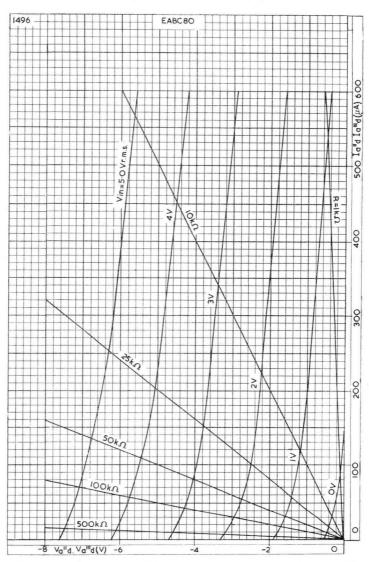
RECTIFIED CURRENT PLOTTED AGAINST OUTPUT VOLTAGE WITH INPUT VOLTAGE BETWEEN 0 AND 5V\_{\rm r.m.s.} AS PARAMETER FOR DIODE SECTIONS  $a^{\prime\prime}_d$  AND  $a^{\prime\prime\prime}_d$
