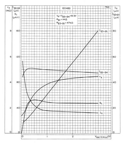
PERFORMANCE CURVES FOR USE AS A FREQUENCY CHANGER  $V_{\rm a} = V_{\rm g2+g4} = 6.3 V \label{eq:varphi}$
