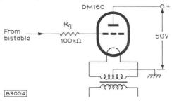
Fig.1 Digital read-out circuit with DM160 connected to negative logic circuit which uses bistables equipped with p-n-p transistors. The 'High' output level of the bistable may vary between 0V and -0.3V, and the 'Low' level between -3V and -6.8V.
