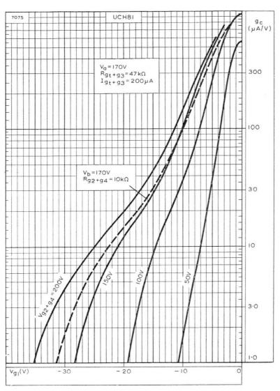
CONVERSION CONDUCTANCE PLOTTED AGAINST CONTROL-GRID VOLTAGE WHEN USED AS A FREQUENCY CHANGER.  $V_a = 170 \text{V}$
