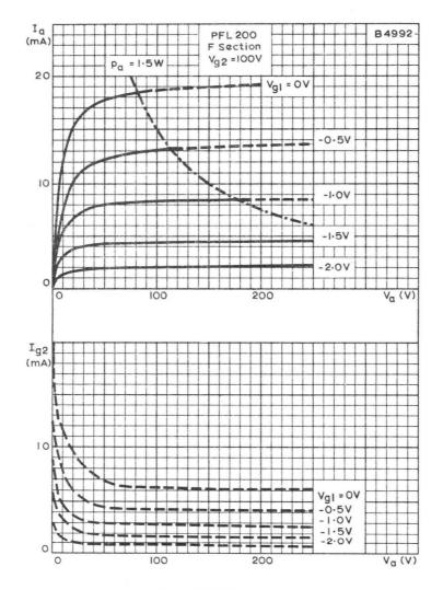
ANODE AND SCREEN-GRID CURRENTS PLOTTED AGAINST ANODE VOLTAGE WITH CONTROL-GRID VOLTAGE AS PARAMETER. V  $_{\rm g2}$  = 100V. F SECTION
