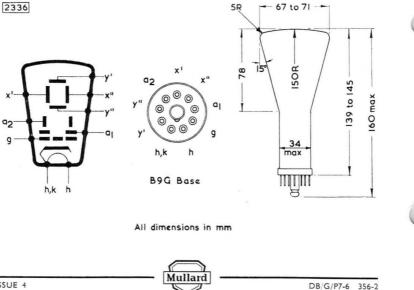
Direct viewing oscilloscope tubes with  $2\frac{3}{4}$  in. diameter screen. Intended for asymmetrical deflection.
