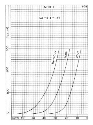
FINAL ANODE CURRENT PLOTTED AGAINST GRID VOLTAGE WITH FIRST ANODE VOLTAGE AS PARAMETER
