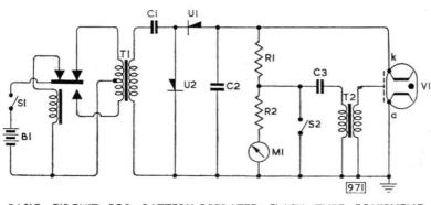
BASIC CIRCUIT FOR BATTERY-OPERATED FLASH TUBE EQUIPMENT
