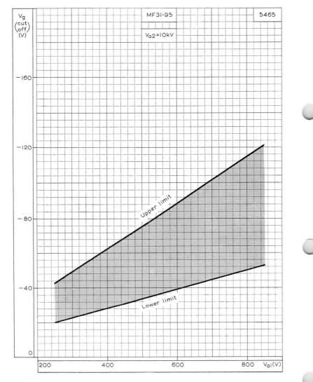
LIMITS OF GRID CUT-OFF VOLTAGE FOR FIRST ANODE VOLTAGES FROM 250V TO 850V.
