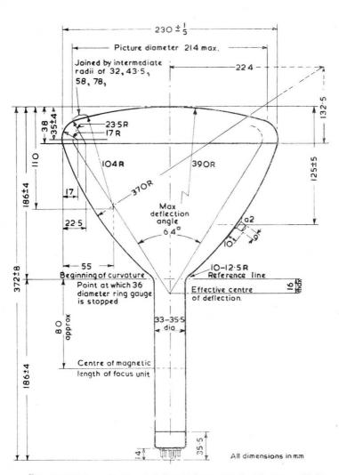
This drawing shows the blown bulb. Some tubes are made with a pressed bulb. A detailed drawing showing the points of difference of the pressed bulb is given on page 4. The base connections are also shown on that page. [2512]
