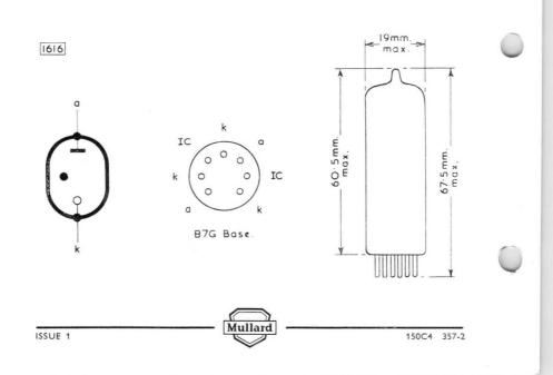
Neon-filled two-electrode tube intended for use as a voltage stabiliser.
