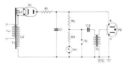
BASIC CIRCUIT FOR MAINS-OPERATED FLASH TUBE EQUIPMENT
