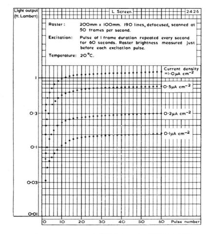
BUILD-UP CHARACTERISTIC OF TYPE 'L' LUMINESCENT SCREEN; REPEATED PULSE EXCITATION. E.H.T.=15kV.
