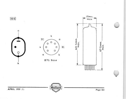
150Volt gas-filled stabiliser with current range of 5.0 to 30mA.
