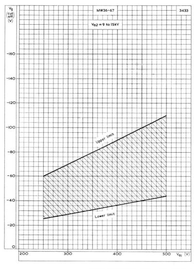
LIMITS OF GRID CUT-OFF VOLTAGE FOR FIRST ANODE VOLTAGES FROM 250 TO 500V
