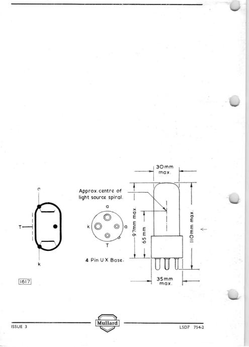
Cold cathode Xenon-filled discharge tube for use in studio or portable photo-flash equipment. Designed for operation with an anode voltage of 1.0 kV.
