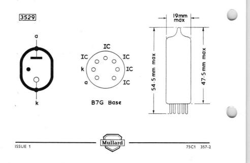
75 Volt gas-filled stabiliser with a current range of 2.0 to 60mA.
