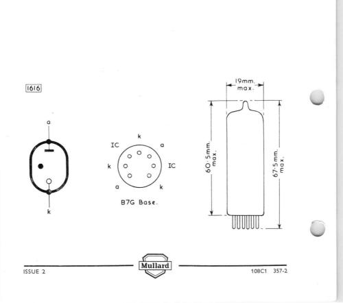
150 volt gas-filled voltage stabiliser with a current range of 5 to 15mA.
