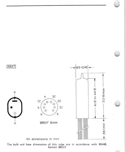
**Note:** Direct soldered connections to the leads of the tube must be at least 5mm from the seal and any bending of the leads must be at least 1.5mm from the seal.
