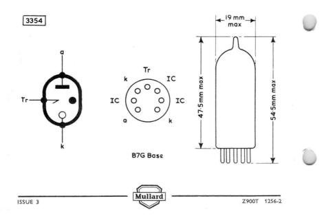
Cold cathode inert gas-filled tube suitable for direct operation from 117V a.c. supplies. The tube is ignited by a positive trigger potential and is primarily intended for on-off relay applications.
