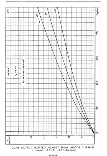
MW43-67 Direct viewing television tube with 17-in. diagonal rectangular metal-backed grey-glass screen. Primarily intended for use as a television studio monitor tube.
