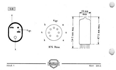
108Volt gas-filled stabiliser with current range 5.0 to 30mA.
