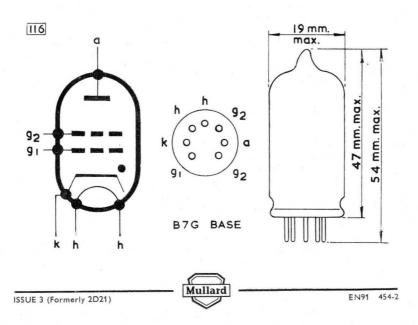
Tetrode inert gas-filled thyratron with negative control characteristic. Primarily designed for use in relay or grid-controlled rectifier circuits.
