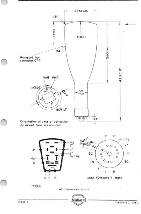
Direct viewing oscilloscope tubes with 5-in. diameter screen. These tubes are fitted with a post-deflection accelerator.
