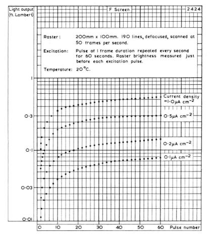
BUILD-UP CHARACTERISTIC OF TYPE 'F' LUMINESCENT SCREEN; REPEATED PULSE EXCITATION E.H.T.=10kV
