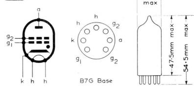
The bulb and base dimensions of this valve are in accordance with BS 448, Section \$B7G\$
