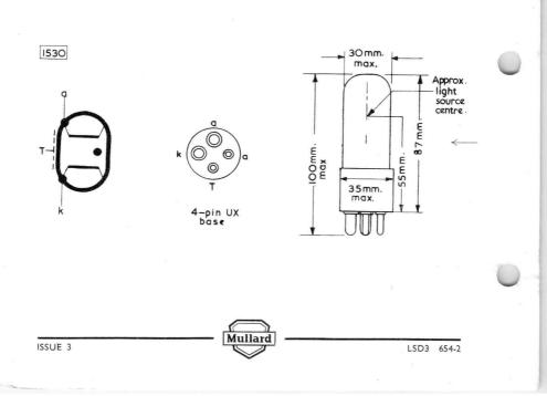
Cold cathode Xenon-filled discharge tube for use in studio photography. A modelling lamp may be inserted within the envelope for use while posing the subject.
