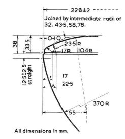
The pressed bulb has the same dimensions as the blown bulb (page 3) apart from the differences shown in the detailed drawing above.
