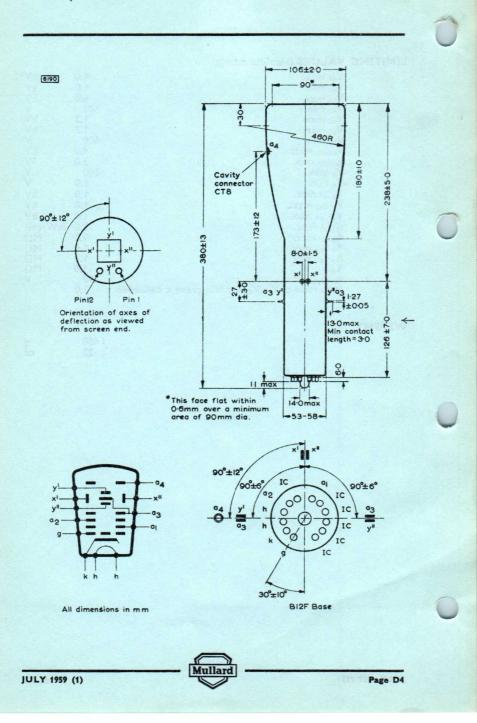
Direct viewing radar tube with 9-in. diameter flatfaced metal-backed screen primarily intended for use in P.P.I. applications. MB22-75 MF22-75
