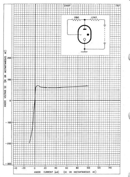
AVERAGE ANODE CHARACTERISTIC WHEN OPERATED AS A RECTIFIER
