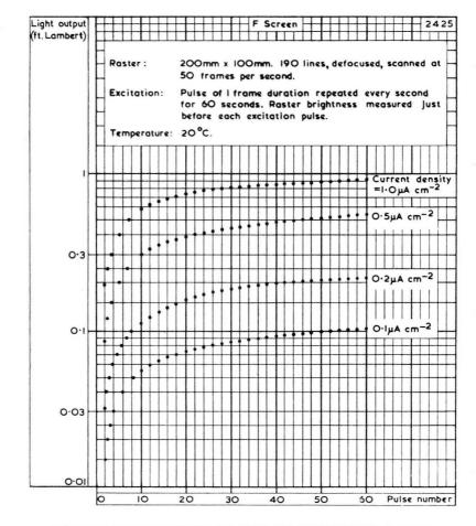
BUILD-UP CHARACTERISTIC OF TYPE 'F' LUMINESCENT SCREEN; REPEATED PULSE EXCITATION E.H.T.=15kV
