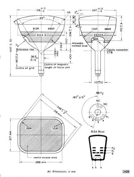
The indicated radius of curvature of the faceplate is not an exact but an average value
