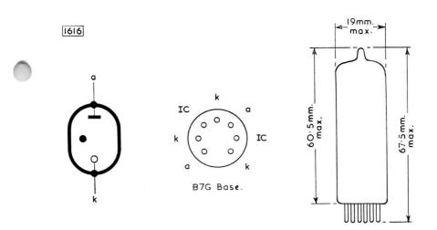
The bulb and base dimensions of this tube are in accordance with BS448 Section B7G
