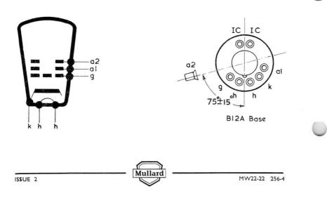
Direct viewing television tube with 9-in. diameter metal-backed screen. Primarily intended for use as a television studio monitor tube.
