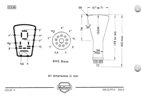
Direct viewing oscilloscope tubes with  $2\frac{3}{4}$  in. diameter screen. Intended for symmetrical deflection.
