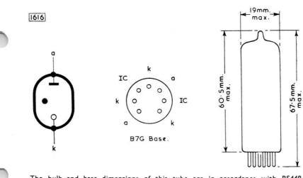
The bulb and base dimensions of this tube are in accordance with BS448 Section B7G
