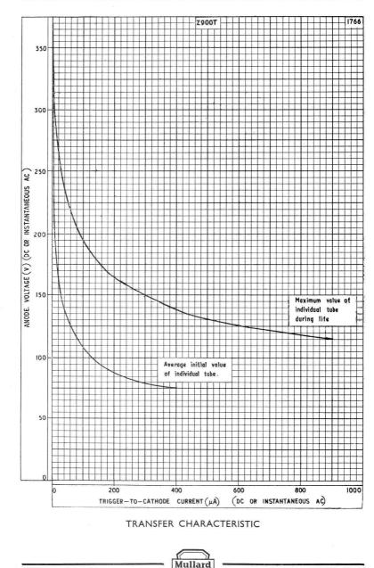
Cold cathode inert-gas filled tube with three electrodes primarily designed for use as a general purpose trigger tube.
