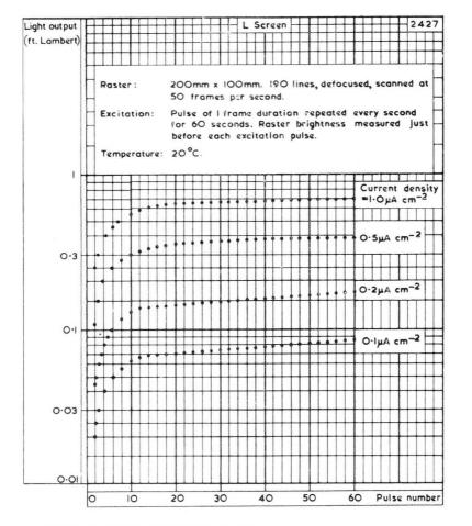
BUILD-UP CHARACTERISTIC OF TYPE 'L' LUMINESCENT SCREEN; REPEATED PULSE EXCITATION. E.H.T.=10kV
