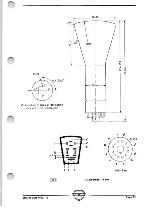
DG7-32 OSCILLOSCOPE TOBE Direct viewing low voltage oscilloscope tube with
