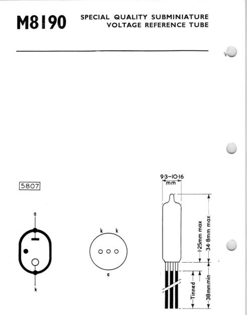
The bulb dimensions of this tube are in accordance with BS448, Section B8D.
