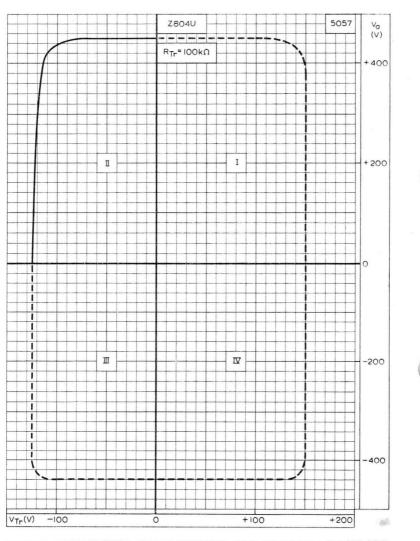
TYPICAL BREAKDOWN CHARACTERISTIC FOR DIFFERENT ELECTRODE POLARITIES
