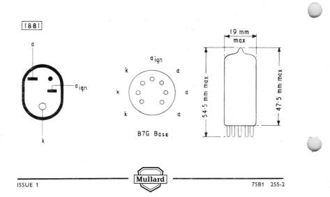
75 Volt gas-filled stabiliser with a current range of 2.0 to 60mA.
