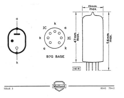
Gas-filled two-electrode tube intended for use as a voltage reference.
