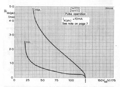
COMBINED PEAK PROBE CURRENT TO ALL NON-CONDUCTING CATHODES
