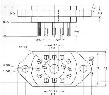
For minimum spacing between adjacent sockets see individual tube data sheets
