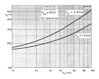
D.C. SUPPLY VOLTAGE PLOTTED AGAINST ANODE LOAD RESISTOR
