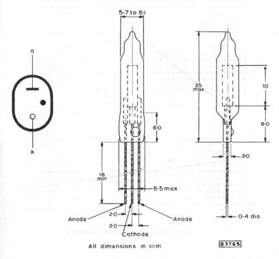
Due to the small physical size of the device, code number stamping has not been possible, therefore for recognition purposes a yellow dot has been painted on the side of the envelope.
