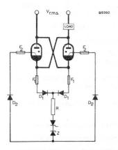
Figure 2:- Anode excitation (common thyristor)
