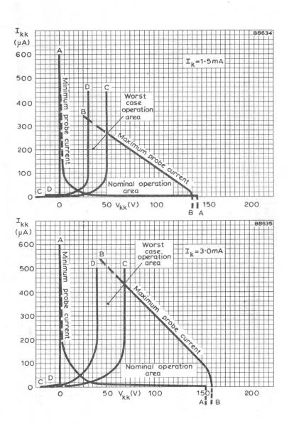
PROBE CURRENTS TO INDIVIDUAL NON-CONDUCTING CATHODES
