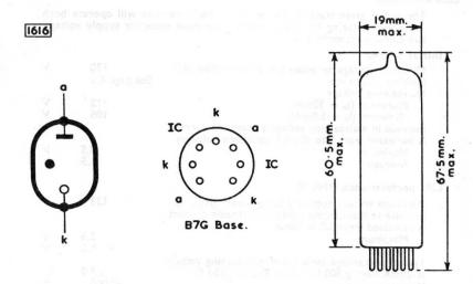
The bulb and base dimensions of this tube are in accordance with BS448,
