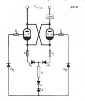
Fig. 2. Anode excitation (Common thyristor)
