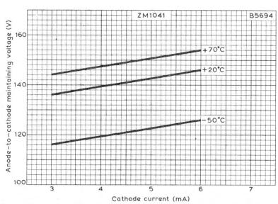
ANODE-TO-CATHODE MAINTAINING VOLTAGE PLOTTED AGAINST CATHODE CURRENT WITH AMBIENT TEMPERATURE AS PARAMETER
