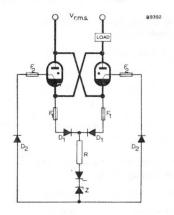
Figure 2:- Anode excitation (common thyristor)
