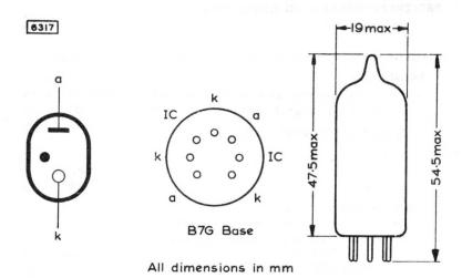
The bulb and base dimensions of this tube are in accordance with BS448, Section B7G.
