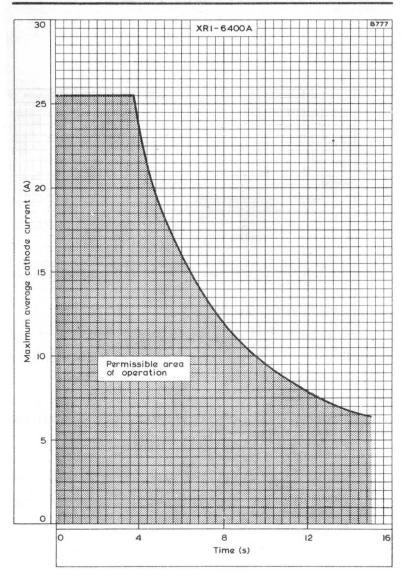
This curve shows the maximum number of seconds in any fifteen second period for which a given average current may be drawn from a sinusoidal supply.
