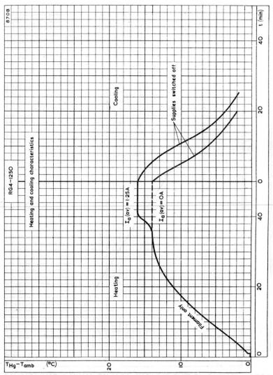
Time required for cathode to reach operating temperature=1 min.
