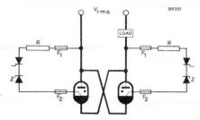
The "Min. peak ignitor voltage for ignition", must not be interpreted as the instantaneous value of mains voltage at the instant of ignition, but as the voltage measured between the ignitor lead-in and cathode. The values of the resistors in the ignition circuit and the level of supply voltage should be chosen so that the prescribed value of voltage is applied to the ignitor.
