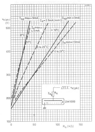
RELATIONSHIP BETWEEN PULSE SUPPLY VOLTAGE AND ANODE RESISTOR
