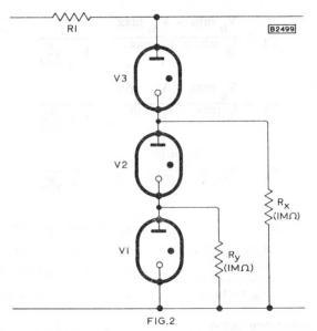
If the resistors  $R_y$  and  $R_x$  cannot be considered as being large compared to the tube load, the conditions applied to each tube must be considered in its own merits as an extension of the basic circuit given in 5.1.
