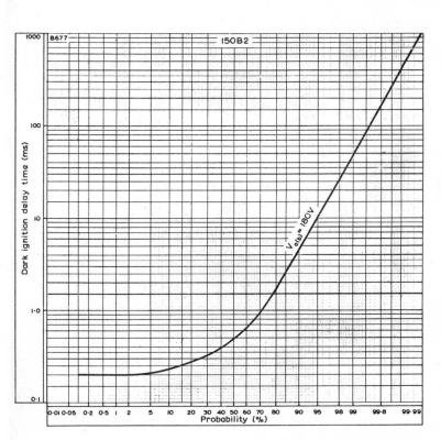
CUMULATIVE DISTRIBUTION OF DARK IGNITION DELAY TIME This curve shows the probability that a tube will ignite in less than the time shown. This will be to some extent dependent on the supply voltage. In general an increase in the supply voltage will reduce the ignition delay time.
