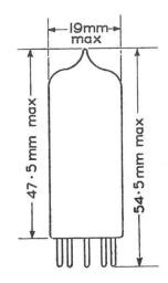
The bulb and base dimensions of this tube are in accordance with BS448, Section B7G.
