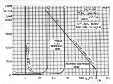
PEAK PROBE CURRENT TO INDIVIDUAL NON-CONDUCTING CATHODES
