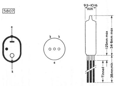
The bulb dimensions of this tube are in accordance with BS448, Section B8D.
