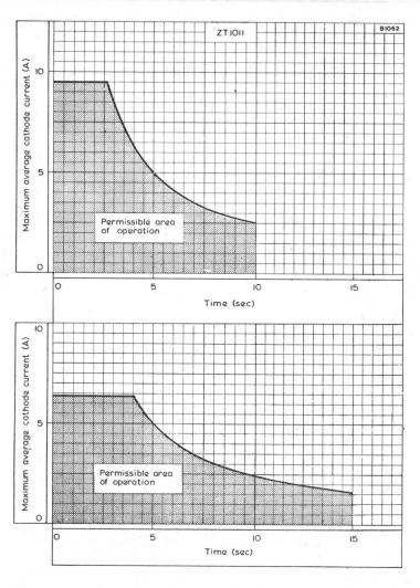
The top curve shows the maximum number of seconds in any 10 second period for which a given average current may be drawn from a sinusoidal supply if the peak voltage applied to the valve is less than 1.25kV. The bottom curve shows the maximum number of seconds in any 15 second period for which a given average current may be drawn from a sinusoidal supply if the applied peak voltage lies between 1.25 and 1.5kV.
