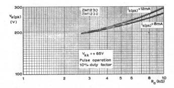
PEAK SUPPLY VOLTAGE PLOTTED AGAINST ANODE LOAD RESISTOR
