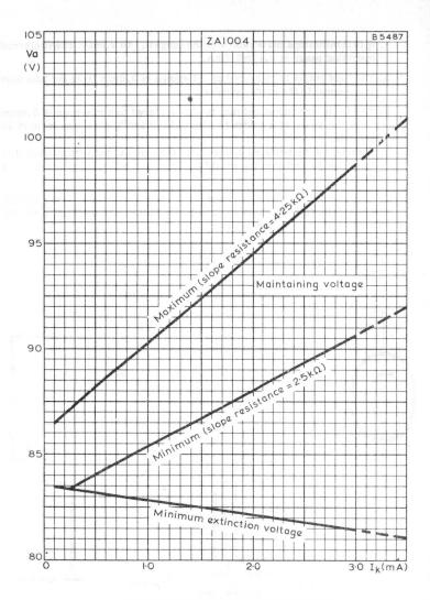
ANODE VOLTAGE CHARACTERISTICS
