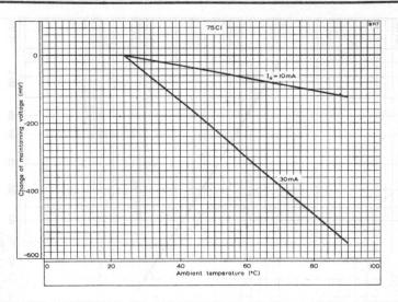
AVERAGE VARIATION OF MAINTAINING VOLTAGE WITH AMBIENT TEMPERATURE
