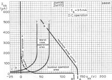
PROBE CURRENT TO INDIVIDUAL NON-CONDUCTING CATHODES
