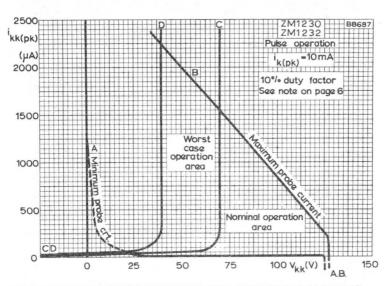
PEAK PROBE CURRENT TO INDIVIDUAL NON-CONDUCTING CATHODES
