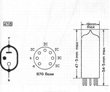
The bulb and base dimensions of this valve are in accordance with BS448, Section B7G
