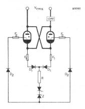
Figure 2:- Anode excitation (Common thyristor)
