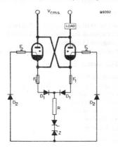
Fig.2: Anode excitation (Common thyristor)
