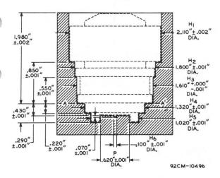
SURFACE A-A' IS FLAT WITHIN 0.0005" PEAK TO VALLEY AND IS PERPENDICULAR TO THE AXIS OF THE CYLINDRICAL HOLES WITHIN 0.00025".
