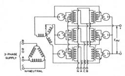
FIG. 6 SERIES THREE-PHASE (QUADRATURE OPERATION)
