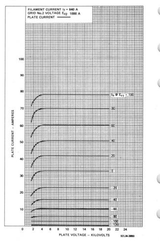
TYPICAL PLATE CHARACTERISTIC (E<sub>c2</sub> = 1000 V) (Type 4648)
