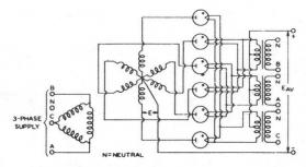
FIG. 8 HALF-WAVE SIX-PHASE (QUADRATURE OPERATION)
