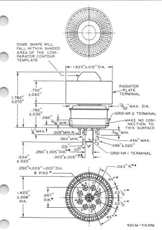
GRID-No.! PLUG DIMENSIONS ARE MEASURED BY THE USE OF THE SERIES OF GAUGES SHOWN IN SKETCHES  $\mathbf{G}_1$  AND  $\mathbf{G}_2$ . IN THE FOLLOWING INSTRUCTIONS FOR THE USE OF THESE GAUGES, "GO" INDICATES THAT THE ENTIRE GRID-No.! PLUG KEY WILL ENTER THE GAUGE; AND "NO-GO" INDICATES THAT THE GRID-No.! PLUG KEY WILL NOT ENTER THE GAUGE MORE THAN I/16". INSTRUCTIONS FOR THE USE OF THE GAUGES FOLLOW:
