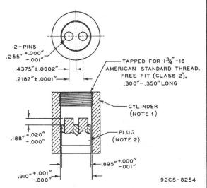
NOTE 1: TAPPED SECTION OF CYLINDER MUST BE CONCENTRIC
