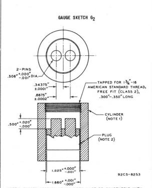
NOTE 1: TAPPED SECTION OF CYLINDER MUST BE CONCENTRIC WITH UNTAPPED SECTION OF CYLINDER WITHIN .002".
