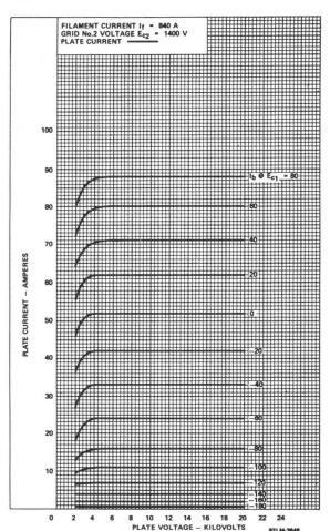
TYPICAL PLATE CHARACTERISTICS (E<sub>c2</sub> = 1400 V) (Type 4648)
