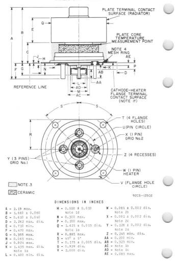
Note I: Concentricity between the various diameters on the major tube axis is such that the tube will enter a gauge having suitably spaced concentric apertures and posts of the following diameters:
