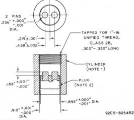
NOTE 1: TAPPED SECTION OF CYLINDER MUST BE CONCENTRIC WITH UNTAPPED SECTION OF CYLINDER WITHIN .002".
