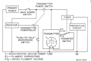
FIG.4 - BASIC RECEIVER-TRANSMITTER WITH AUXILIARY
