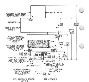
ELECTRODE-TEMPERATURE MEASUREMENT POINT
