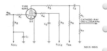
C<sub>1</sub>: 0.1 \(\mu f\), 600 \(\mu\) dc C<sub>2</sub>: 2 \(\mu f\), 600 \(\mu\) dc C<sub>3</sub>: 0.25 \(\mu f\), 5000 \(\mu\) dc
