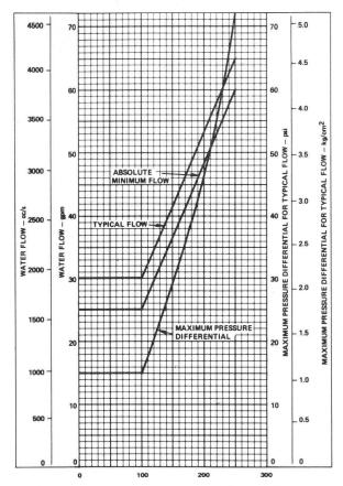
AVERAGE PLATE DISSIPATION - KILOWATTS
