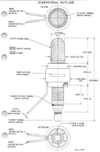
NOTE: Recommended direction of anode coolant flow: Duct #1 is "IN" and Duct #2 is "OUT" when tube is operated with Output Ceramic Dome UP. With Output Ceramic Dome DOWN, the flow should be reversed.
