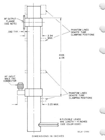
Note: RF output flange requires use of a transition piece (Waveline Type 60083, or equivalent) if matching to standard waveguide flange.
