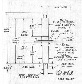
MAXIMUM ECCENTRICITY OF CENTER LINE (AXIS) OF PLATE TERMINAL OR GRID-TERMINAL FLANGE WITH RESPECT TO THE CENTER LINE (AXIS) OF THE CATHODE TERMINAL IS 0.010".
