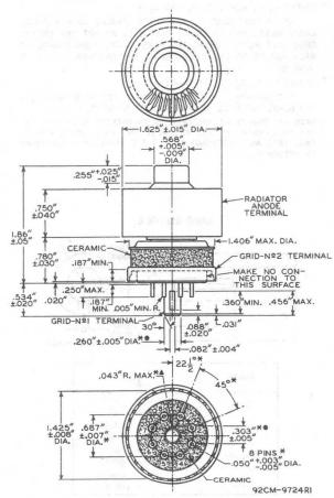
GRID-No.1-PLUG DIMENSIONS ARE MEASURED BY THE USE OF THE SERIES OF GAUGES SHOWN IN SKETCHES  $\mathsf{G}_1$  AND  $\mathsf{G}_2$ . IN THE FOLLOWING INSTRUCTIONS FOR THE USE OF THESE GAUGES "GO" INDICATES THAT THE ENTIRE GRID-No.1-PLUG KEY WILL ENTER THE GAUGE; AND "NO-GO" INDICATES THAT THE GRID-No.1-PLUG KEY WILL ENTER THE GAUGE MORE THAN 1/16". INSTRUCTIONS FOR THE USE OF THE GAUGES FOLLOW:
