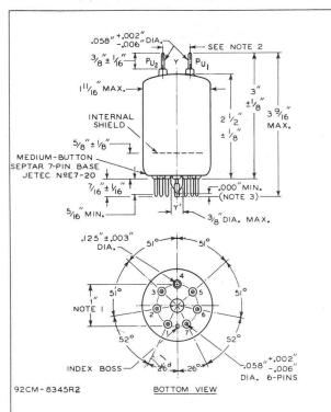
THE REFERENCE AXIS YY' IS DEFINED AS THE AXIS OF THE BASE-PIN GAUGE DESCRIBED IN NOTE 1.
