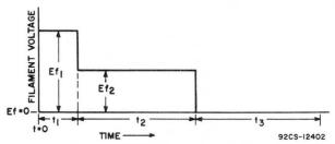
FIG.3 - FILAMENT VOLTAGE WAVE FORM
