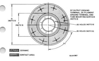
DETAIL OF RF INPUT CATHODE AND RF GRID NO. 1 TERMI-NAL, CONTACT SURFACES AND DC GRID NO. 1 TERMINAL
