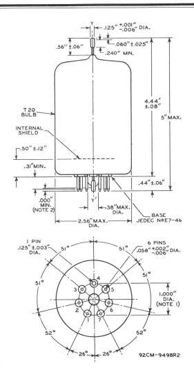
THE REFERENCE AXIS Y-Y' IS DEFINED AS THE AXIS OF THE BASE PIN GAUGE DESCRIBED IN NOTE I:
