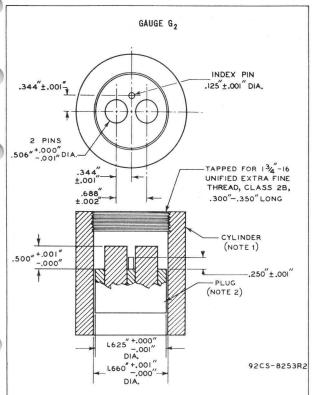
NOTE 1: TAPPED SECTION OF CYLINDER MUST BE CONCENTRIC WITH UNTAPPED SECTION OF CYLINDER WITHIN .002". NOTE 2: PLUG SIDES & PIN SIDES MUST BE PARALLEL WITHIN .001".
