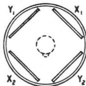
ORIENTATION OF THE DEFLECTOR PLATES AS VIEWED FROM THE SCREEN END
