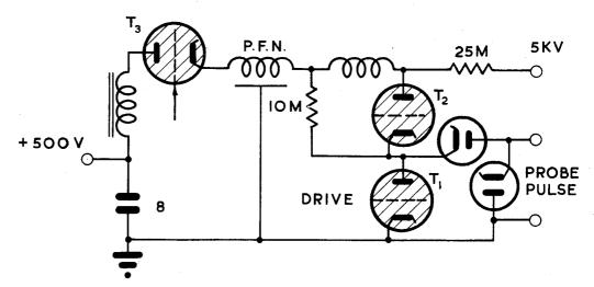
A probe pulse is applied to the Anode of the thyratron T1 under investigation. Thyratron T2 isolates the pulse forming network from the probing pulse. Thyratron T3 prevents the charging of the network until this is desired. The circuit possesses no dissipative elements, inevitable losses are made good from the 500%, supply.
