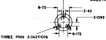
VIEW OF UNDERSIDE OF BASE ALL DIMENSIONS IN MILLIMETRES
