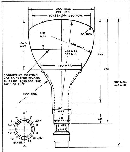
NOTES. I. VIEWING THE SCREEN OF THE TUBE WITH BASE SPIGOT UPPERMOST, A POSITIVE VOLTAGE. APPLIED TO THE TERMINAL XI SHALL DEFLECT THE SPOT TO THE RIGHT, AND A POSITIVE VOLTAGE APPLIED TO THE TERMINAL YI SHALL DEFLECT THE SPOT DOWNWARDS.
