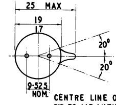
CENTRE LINE OF SEALING-OFF PIP TO LIE WITHIN THESE LIMITS. DIA. OF BASE OF PIP NOT TO EXCEED 5 MM.
