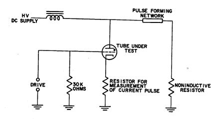
Figure 2. Test circuit.
