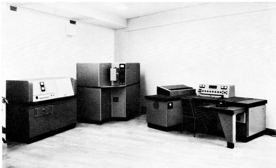
The "Spectrovide" emission spectrometer combined with excitation source and measuring console to form a direct reading spectrochemical installation.
