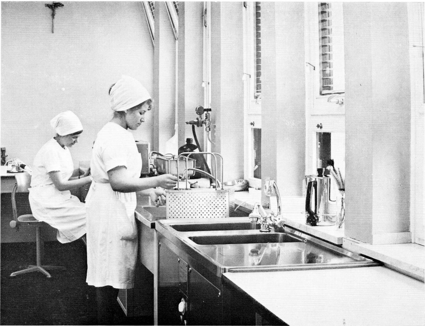
Ultrasonic cleaning equipment in a hospital.
