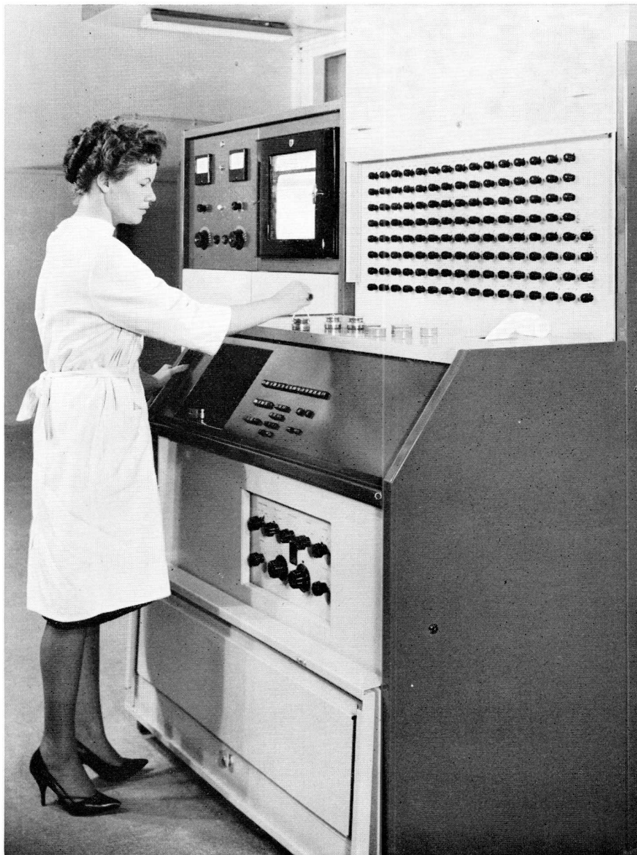
Automatic spectrometer, type PW 1212.
