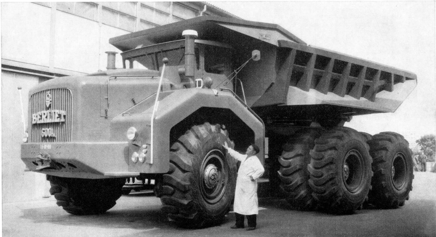
This huge truck is built by Messrs. Benne Marrel, of Saint-Etienne, France. For the welding work Philips low-hydrogen electrodes and rutile electrodes were used.
