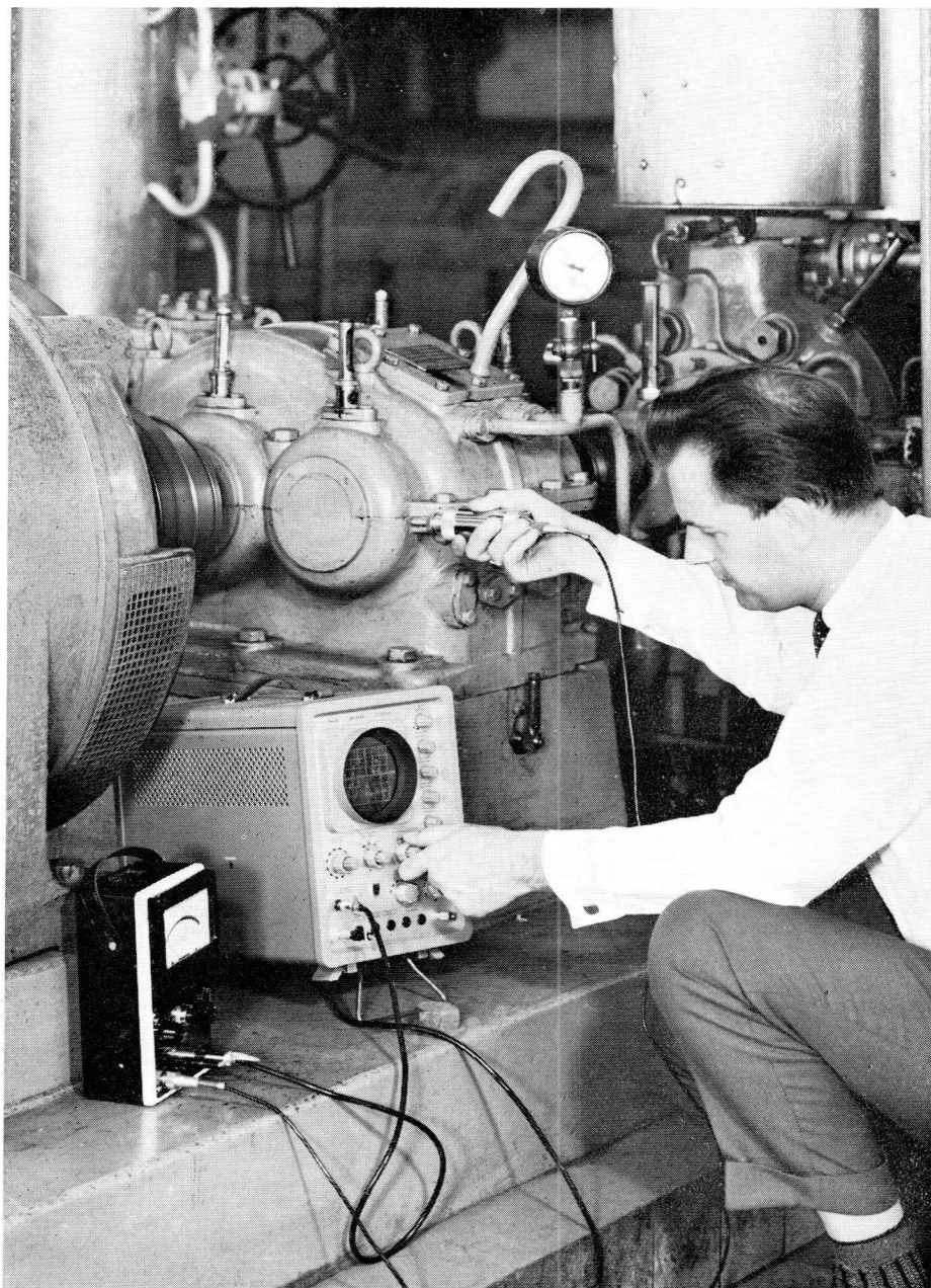
Vibration measurement with transducer, direct reading vibration meter and oscilloscope.
