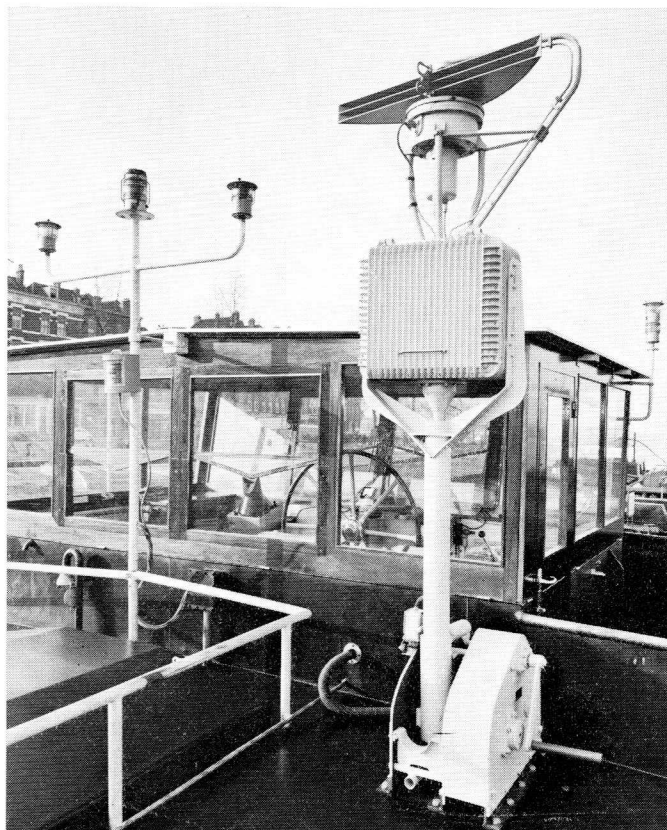
Antenna, mounted directly to the watertight transmitter/receiver cabinet of a 9 mm high-definition radar installation on board an inland water tanker.
