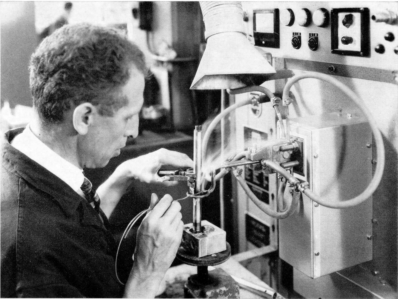
Brazing with a 12 kW h.f. generator.
