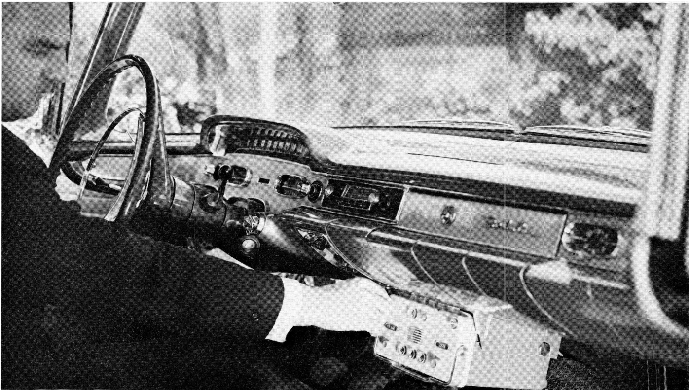
Semaphore receiver, in this photograph used in a car.
