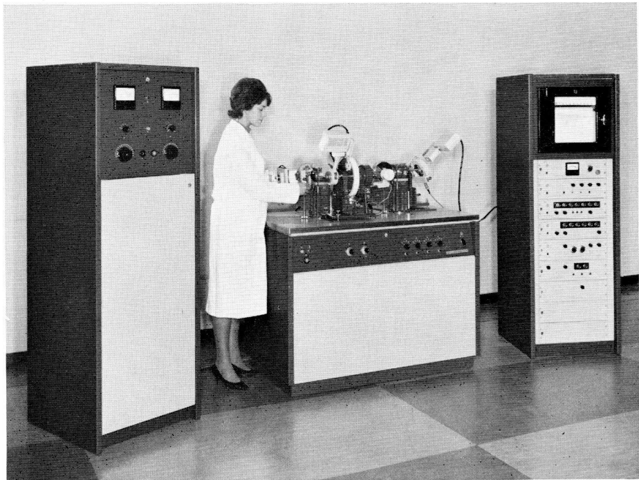
Complete instrumentation for X-ray diffraction and diffractometry based on the X-ray diffraction generator, type PW 1310 equipped with two tube shields. On the left separate control cabinet type PW 1320. For X-ray diffractometry the transistorized electronic circuit panel, type PW 1352/00 is used with the generator.
