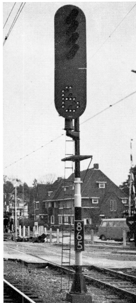
Type Velsin route or speed indicator (photograph by kind permission of Netherlands Railways)
