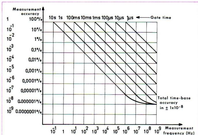
Fig. 4.6. Frequency error as function of gate time,  $\pm 1$  count ambiguity and clock accuracy.
