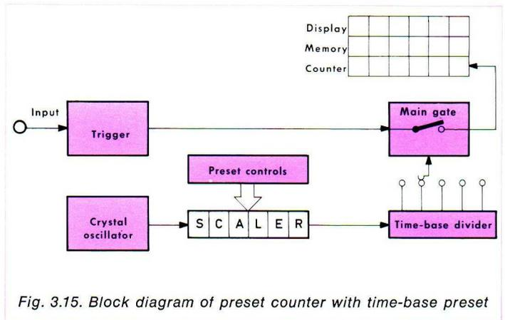
Fig. 3.15. Block diagram of preset counter with time-base preset
