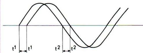
Fig. 2.8. Phase-difference measurement
