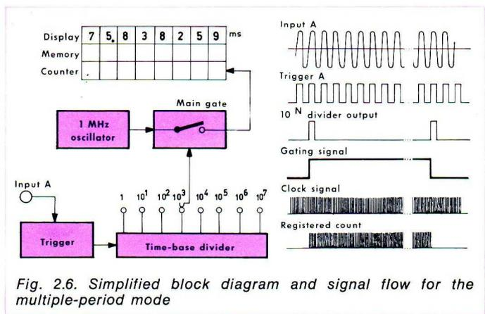
Fig. 2.6. Simplified block diagram and signal flow for the multiple-period mode
