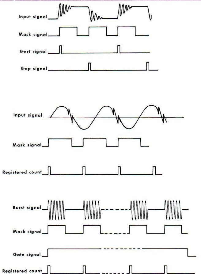
Fig. 4.21a. Pulse-width measurement on a signal with considerable "ringing"
