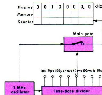
Fig. 2.14. Simplified block diagram for self-check operation
