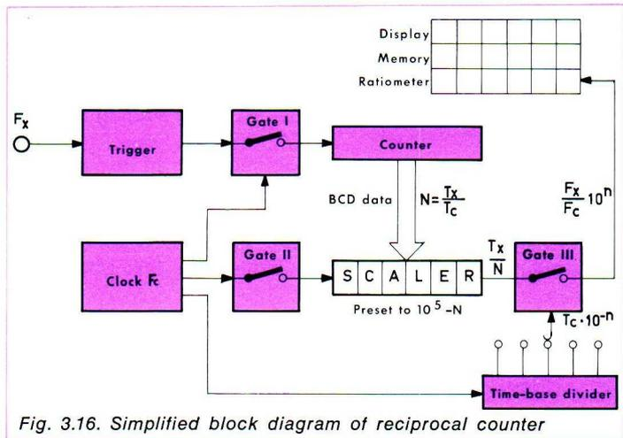
Fig. 3.16. Simplified block diagram of reciprocal counter
