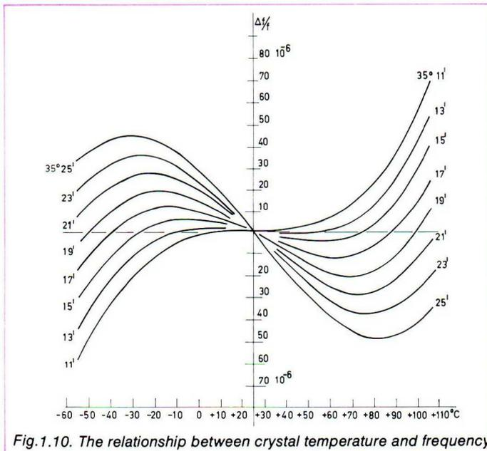
Fig. 1.10. The relationship between crystal temperature and frequency
