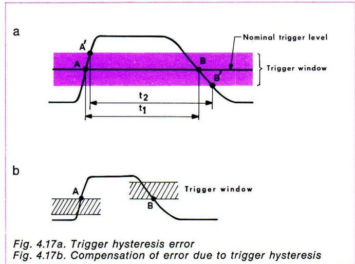
Fig. 4.17a. Trigger hysteresis error
