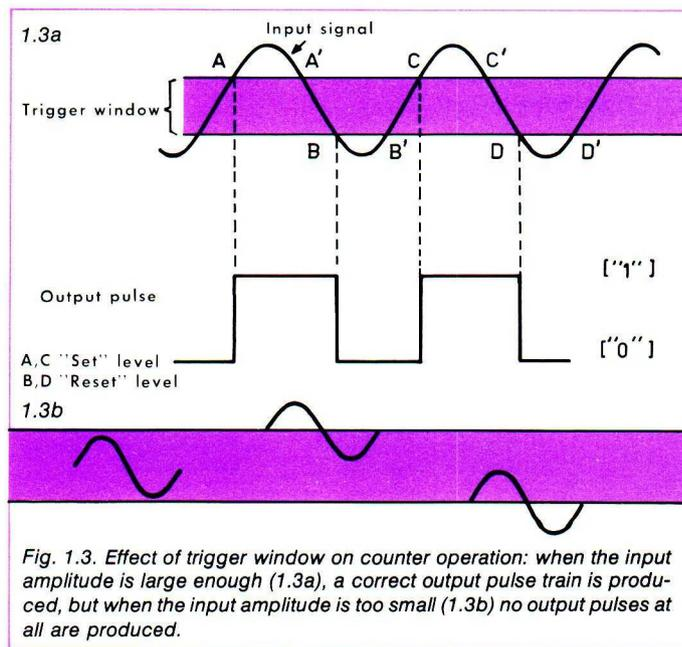
Fig. 1.3. Effect of trigger window on counter operation: when the input amplitude is large enough (1.3a), a correct output pulse train is produced, but when the input amplitude is too small (1.3b) no output pulses at all are produced.
