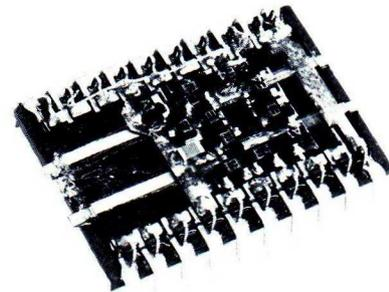
*High-frequency main gate in thin-film technique*
