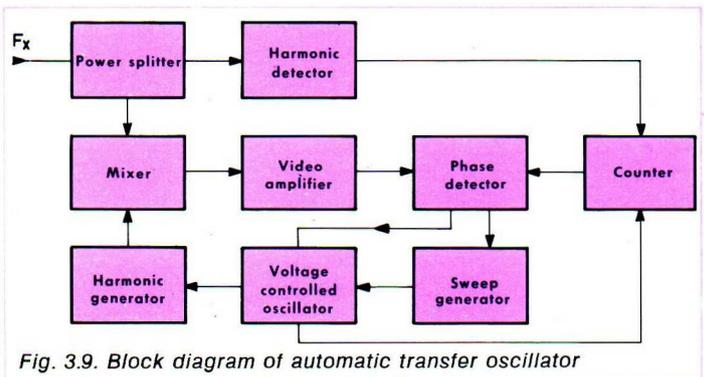
Fig. 3.9. Block diagram of automatic transfer oscillator
