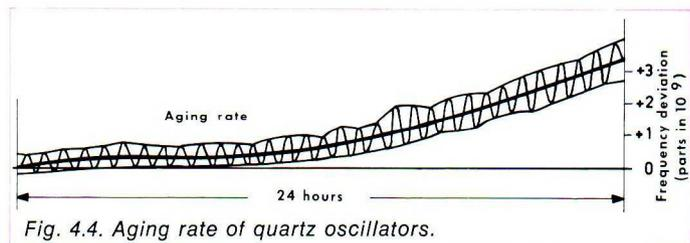
Fig. 4.4. Aging rate of quartz oscillators.
