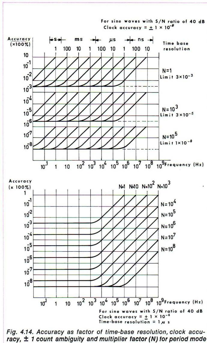
Fig. 4.14. Accuracy as factor of time-base resolution, clock accuracy,  $\pm 1$  count ambiguity and multiplier factor (N) for period mode
