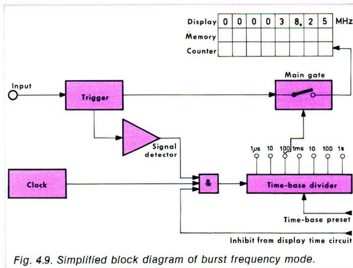
Fig. 4.9. Simplified block diagram of burst frequency mode.
