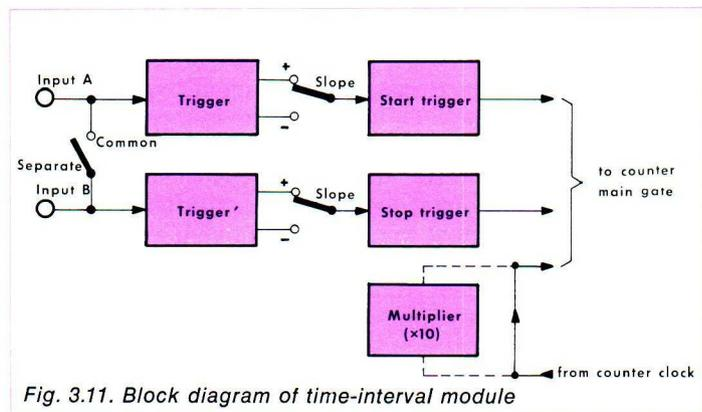
Fig. 3.11. Block diagram of time-interval module
