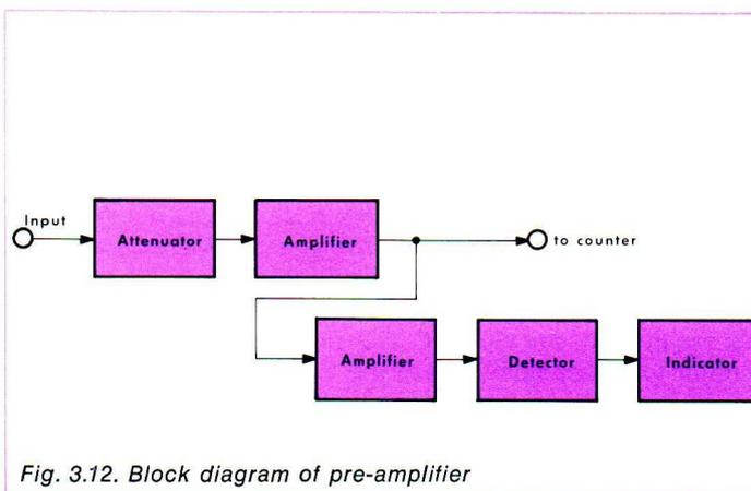
Fig. 3.12. Block diagram of pre-amplifier
