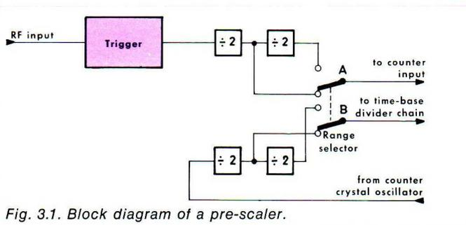
Fig. 3.1. Block diagram of a pre-scaler.
