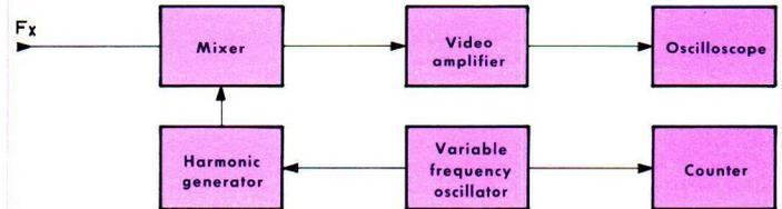
Fig. 3.7. Block diagram of a TO plug-in
