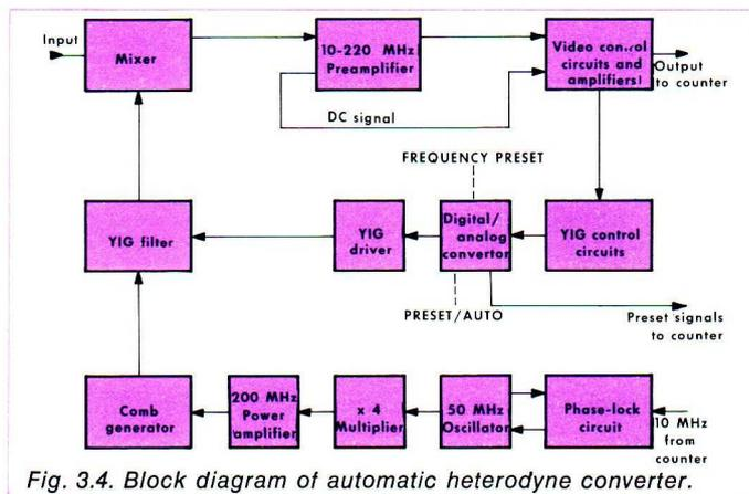
Fig. 3.4. Block diagram of automatic heterodyne converter.
