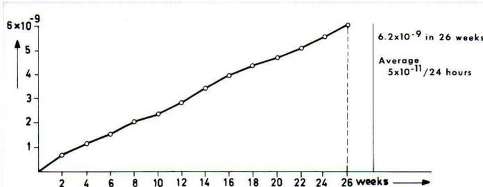
Fig. 4.5. Aging characteristic of Philips PM 9680 crystal oscillator in proportional controlled oven.
