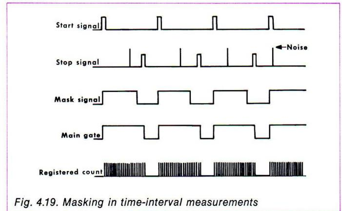
This masking facility is particular useful for measurement of the closing time of a relay, where contact bounce generally gives problems: instead of measuring the correct closing time, most timers will measure only the duration of the first bounce. With the masking circuit, the effect of the bounce time can be eliminated by adjusting the delay to be longer than the bounce period (fig. 4.20).
