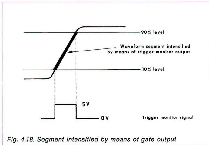
One possible method, used in the PM 6650, is to monitor the time interval to be measured on an oscilloscope screen. The gate signal (representing the time between opening and closing of the main gate) is available at an additional output and may be used for intensifying (Z-axis modulation) the waveform segment over which the time interval is measured (see fig. 4.18.).
