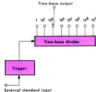
Fig. 2.13. Simplified block diagram for scaler operation
