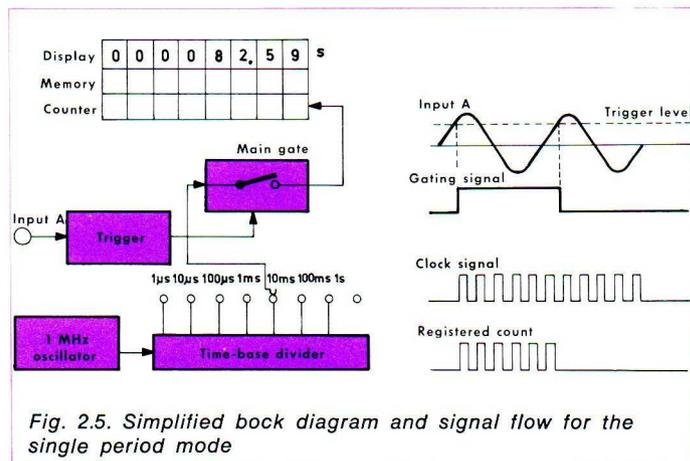
Fig. 2.5. Simplified block diagram and signal flow for the single period mode
