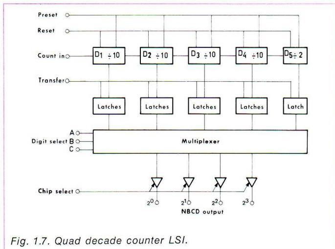
In fact, the dynamic display system described above is more complicated than found in practice, in the interests of clear explanation of the display principle. The memory of a real dynamic display can generally be built up of 4-parallel n-bit shift-register chains. (The "4-parallel" refers to A, B, C and D data, and the n to the number of decades.)
