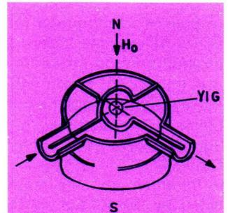
Coupling structure of a single-stage YIG band-pass filter.
