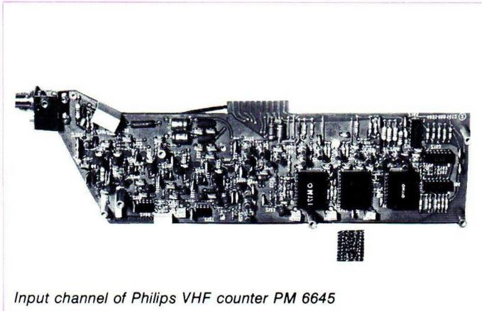
*Input channel of Philips VHF counter PM 6645*
