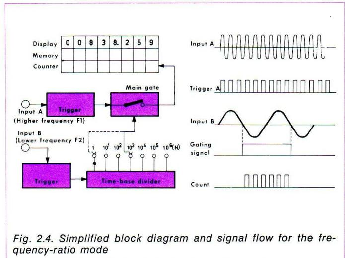
Fig. 2.4. Simplified block diagram and signal flow for the frequency-ratio mode
