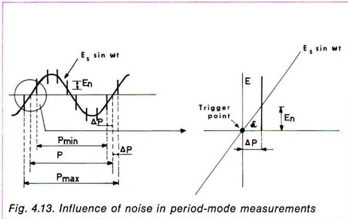
Fig. 4.13. Influence of noise in period-mode measurements
