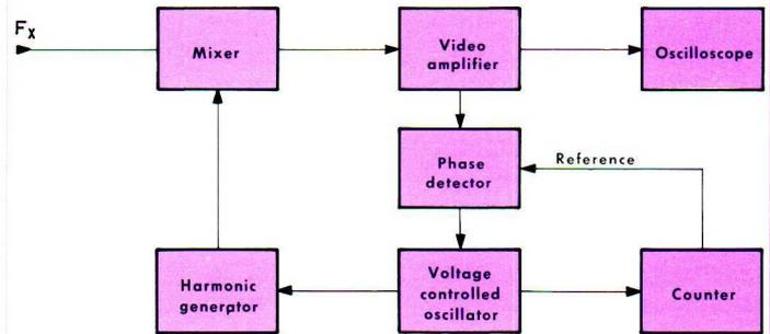
Fig. 3.8. Transfer oscillator with phase-locked loop
