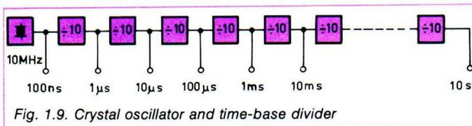
Fig. 1.9. Crystal oscillator and time-base divider
