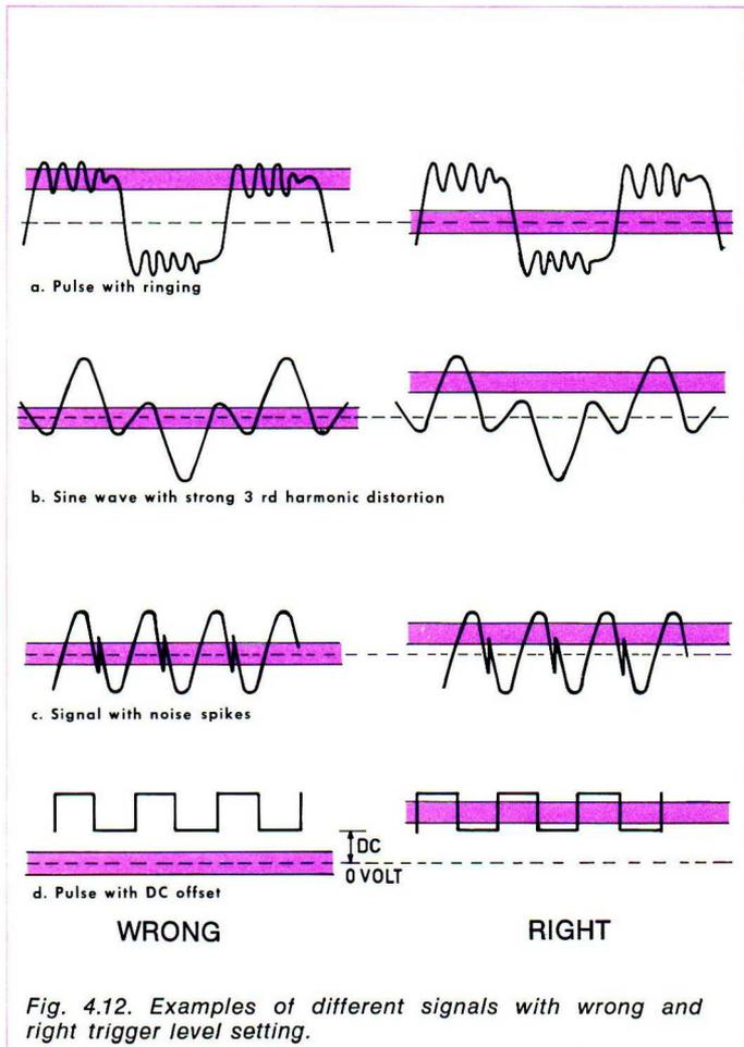
Fig. 4.12. Examples of different signals with wrong and right trigger level setting.
