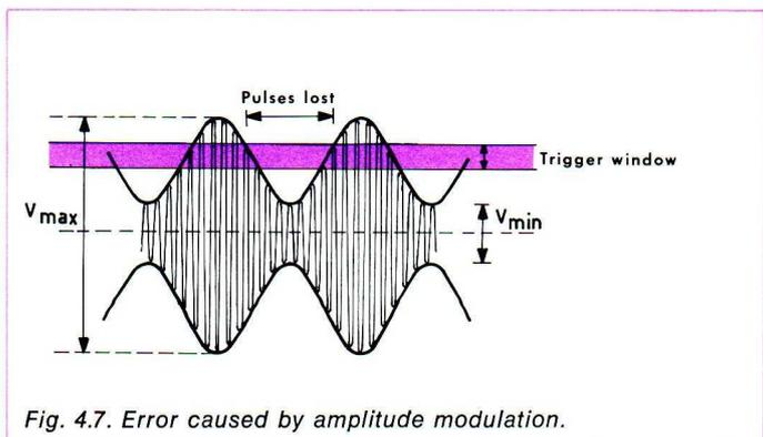
Fig. 4.7. Error caused by amplitude modulation.
