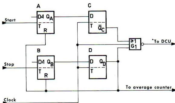
Fig. 4.23. Synchronous gating in the time-interval average mode
