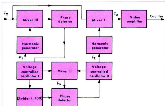
Fig. 3.10. Block diagram of automatic frequency divider
