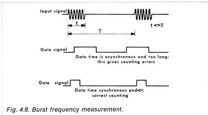
Fig. 4.8. Burst frequency measurement.
