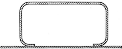
Fig. 179. Sketch of joint unsuitable for spot welding.
