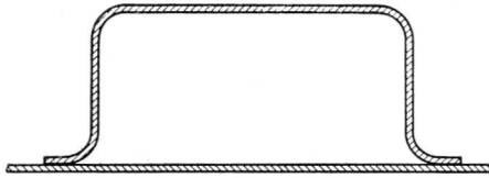
Fig. 180. Sketch of same joint for suitable spot welding.
