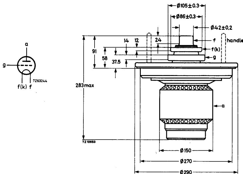
Note: The handles should be removed before switching on the tube.
