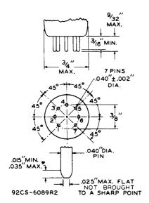
\*This dimension around the periphery of any individual pin may vary within the limits shown.
