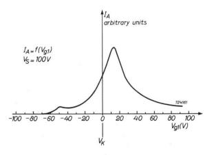
Fig.4. Anode current variation with the adjustment of  $g_1$ .
