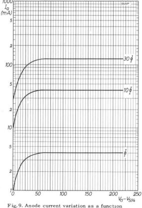
of the voltage between last dynode and anode.
