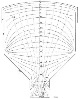
Fig. 3. Electron optical input system.
