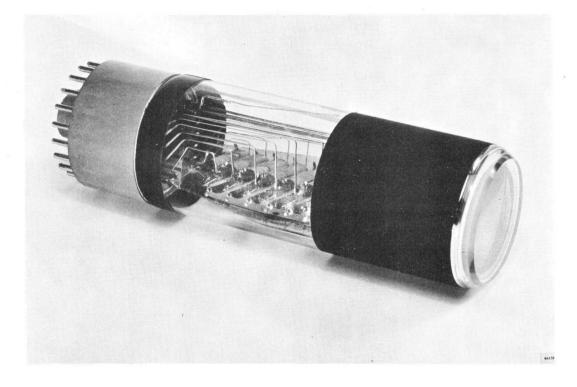
The 56 AVP is 14-stage, very fast, high-gain photomultiplier tube, provided with a caesium-antimony, semi-transparent curved cathode having a diameter of 42 mm. The plane-concave poly-optical window simplifies and improves the optical coupling of scintillator to photocathode. The highly sensitive uniform photocathode has a typical sensitivity of 60  $\mu$ A/lm and a spectral response that lies mainly in the visible region, with its maximum at 4200 Å, as shown in Fig.1, curve A.
