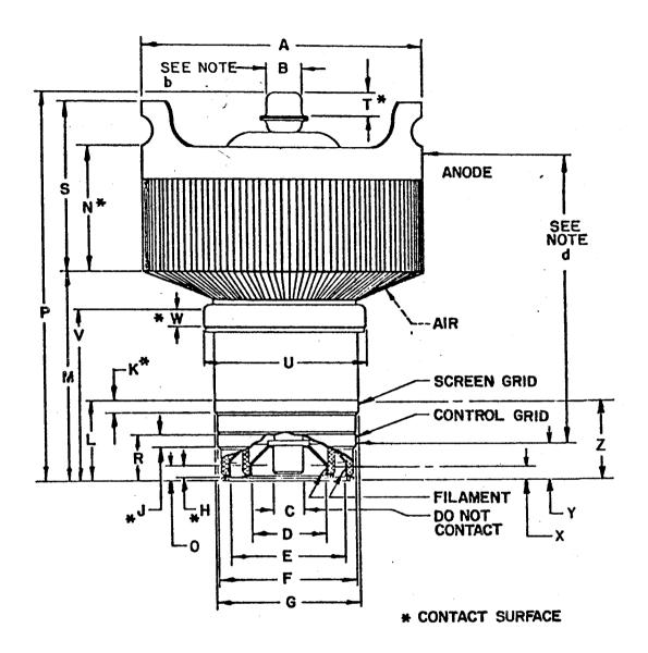
FIGURE 1. Outline drawing of electron tube type 8281.
