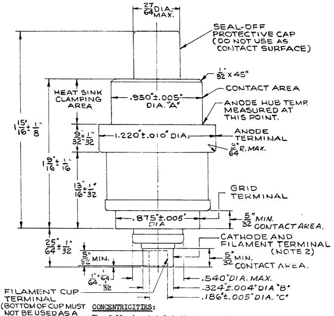
The following total indicator readings are measured with respect to a centerline determined by the centers of the anode terminal and control grid terminal.
