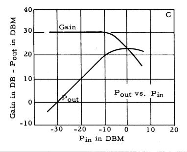
All data shown with magnetic field adjusted for best trans-mission in range of 900 to 1300 gauss and control electrode voltage adjusted for maximum collector current with shell current less than 3 ma.
