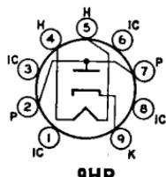
Novar type used as damper tube in horizontal-deflection circuits of color and black-and-white television receivers. Outline section, 30B; requires novar 9-contact socket. Socket terminals 1, 3, 6, and 8 should not be used as tie points. This tube, like other power-handling tubes, should be adequately ventilated.
