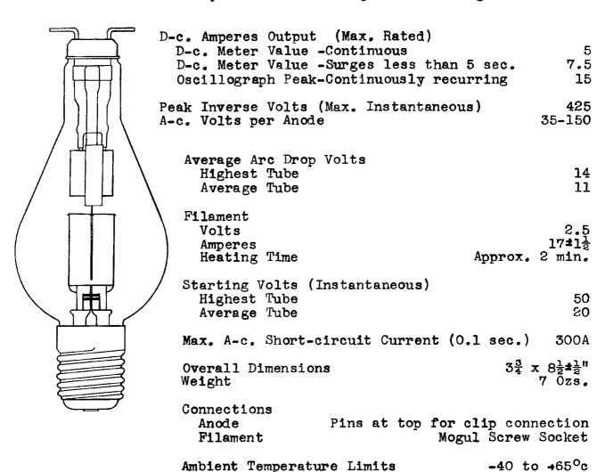
The EL 5B Heavy Duty has a much larger heat shielded cathode than the EL 5B Standard and is designed for service where the load fluctuates violently, or where exceptionally long life is desired. Load and filament voltage may be applied simultaneously without immediate damage, but life is materially shortened by each such cold start.
